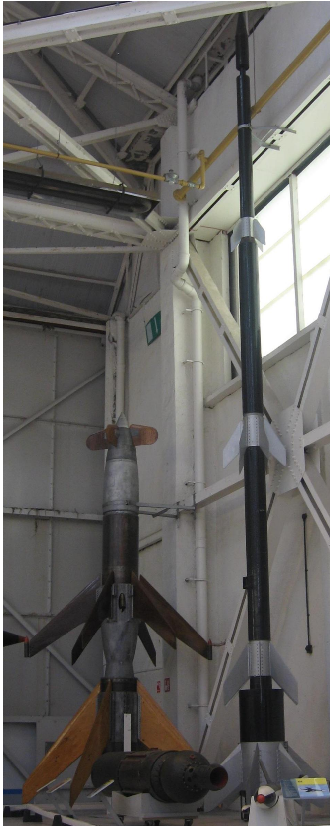
Figure E.260: Rheintochter R1 two-stage solid propellant rocket (left), partial Rheintochter R3 strap-on solid propellant booster (horizontal, center), and Rheinbote four-stage solid propellant rocket (right).
