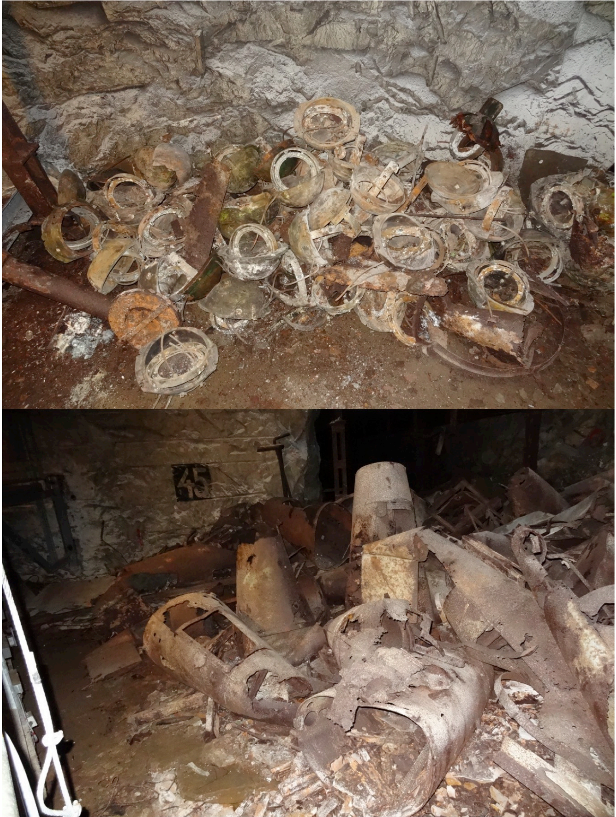
Figure E.59: The Mittelbau tunnel complex in Nordhausen now. In addition to the V-2 (A-4) rocket, the V-1 cruise missile was mass-produced here. Above are housings for V-1 magnetic compasses and below are V-1 tails.
