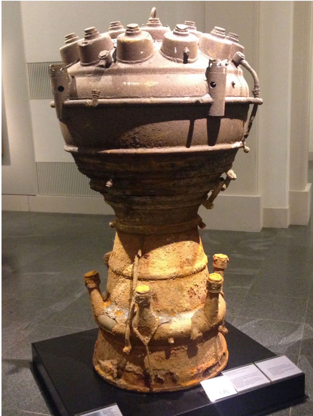
Figure E.48: Standard A-4 rocket engine with propellant injection cups on top.
