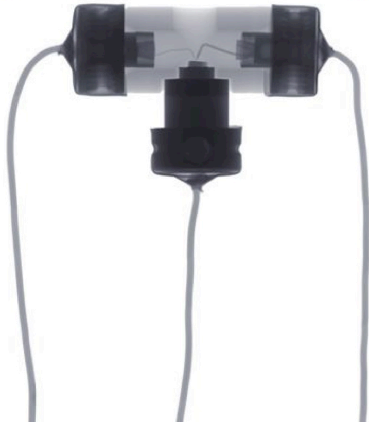
Figure B.50: Heinrich Welker and Herbert Mataré began developing a point-contact transistor in Germany during the war, filed a detailed patent application based on that wartime work on 6 April 1945, and publicly announced their transistor in 1948 in France.
