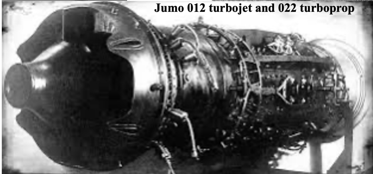
Jumo 022, a.k.a. NK-12, turboprop engine is still in service on the Russian Tupolev Tu-95
