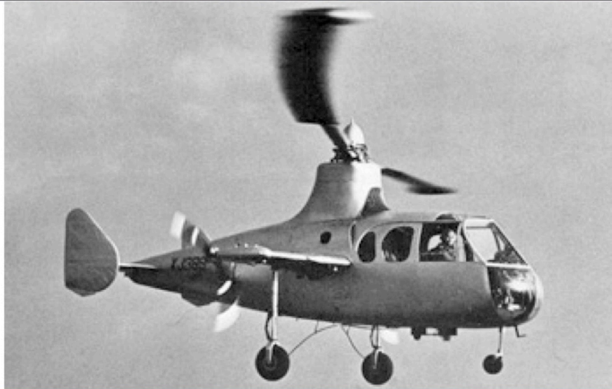
Fairey Jet Gyrodyne with tip-jet rotor (1954) designed by August Stepan and Alexander Czernin
