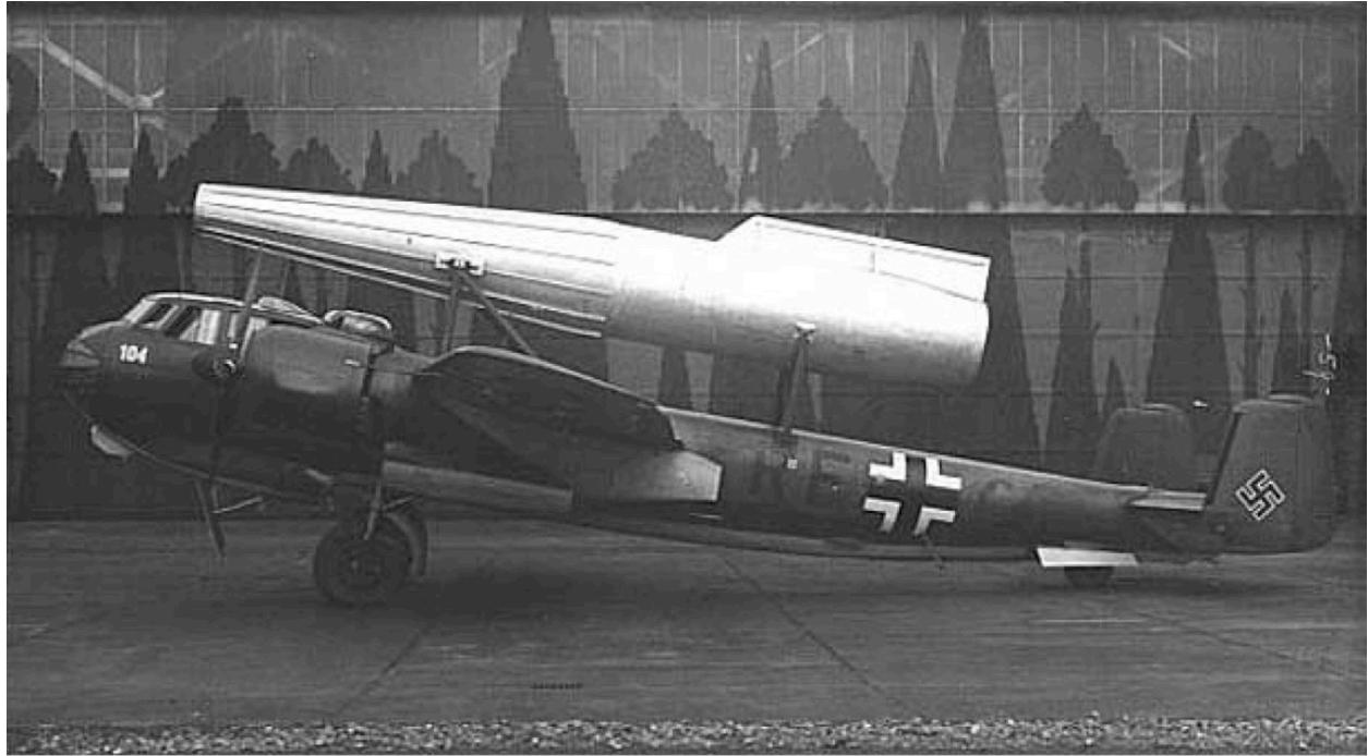
Eugen Sänger's ramjet being tested on a Dornier Do 217 aircraft (1942)
