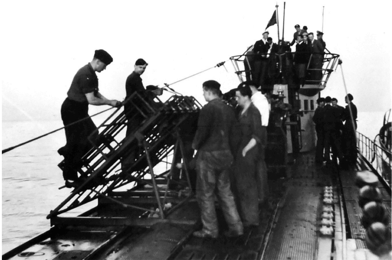
Nebelwerfer rockets launched from U-511 U-boat 12 meters underwater (May 1942)
