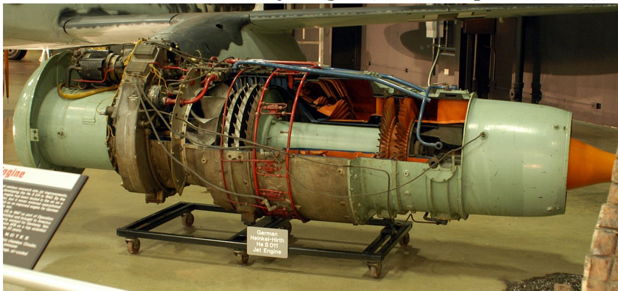
Figure 9.69: Top: Ernst Heinkel and Hans von Ohain celebrating the flight of the first jet aircraft, the Heinkel He 178, in 1939. Bottom: The HeS 011 turbojet engine, developed by von Ohain and Max Adolf Müller (first run September 1943).
