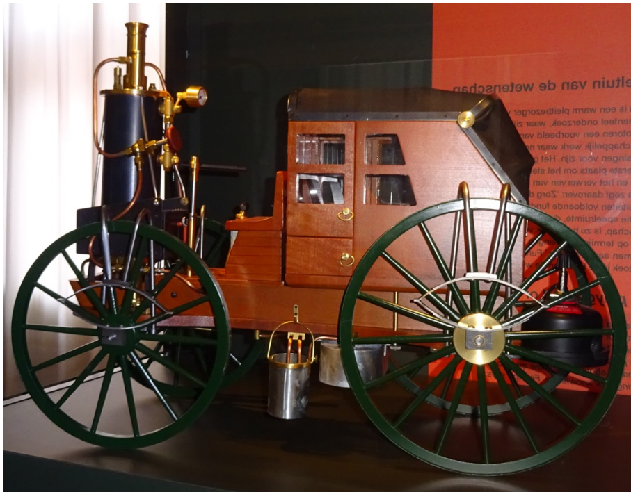
Figure 7.29: Sibrandus Stratingh (Dutch, 1785–1841) and Christopher Becker (German states, 17??–18??) developed and demonstrated a steam-powered car in 1834 (miniature replica shown) and a small electric car in 1835. Becker also created astronomical measuring instruments.
