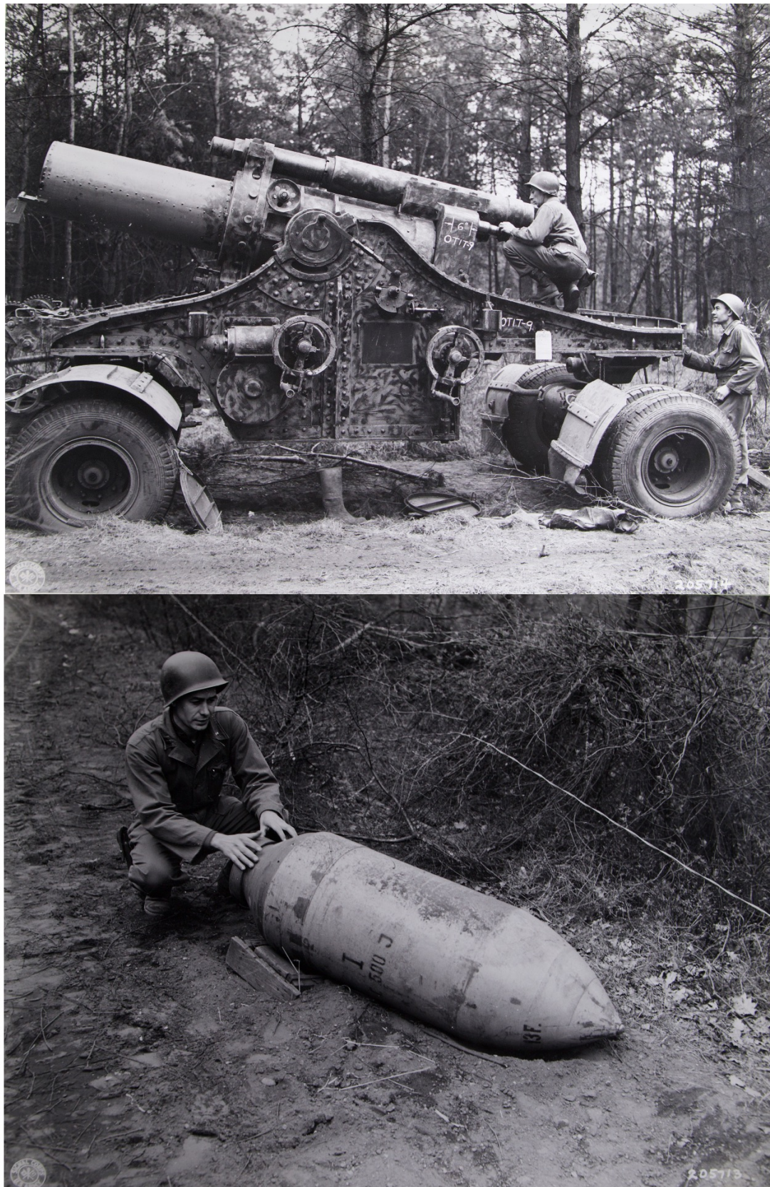
Figure 7.98: Original photo caption: “U.S. Army Ordnance men inspect howitzer-like gun captured by 30th Division units. The gun fires a rocket-type shell 15 inches in diameter, weighing about 1,500 pounds. 4/2/45” [NARA Still Pictures, RG 111 SCA—Records of the Chief Signal Officer. Prints: U.S. Army Signal Corps Photographs of Military Activity During WW II and the Korean Conflict, 1941–1954. Captured German Equipment, German, Box 3344, Book 5, SC 205713, SC 205714.]
