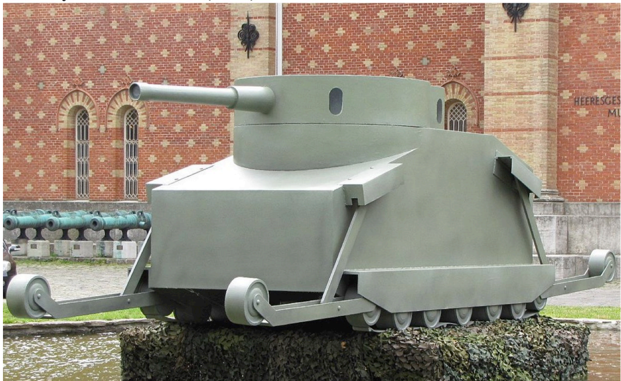
Figure 7.54: In or before 1911, Günther Burstyn invented the first combat tank to incorporate all of the major features of modern tanks. It also had extendable wheeled beams on the front and back to aid in crossing over trenches.
