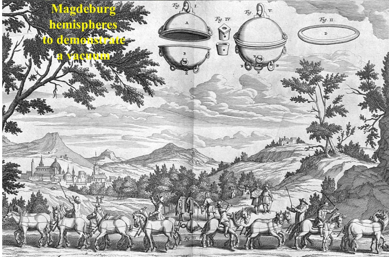
Figure 7.137: Otto von Guericke invented the water barometer, manometer, and air pump, and he also created the “Magdeburg hemispheres” to demonstrate a vacuum.
