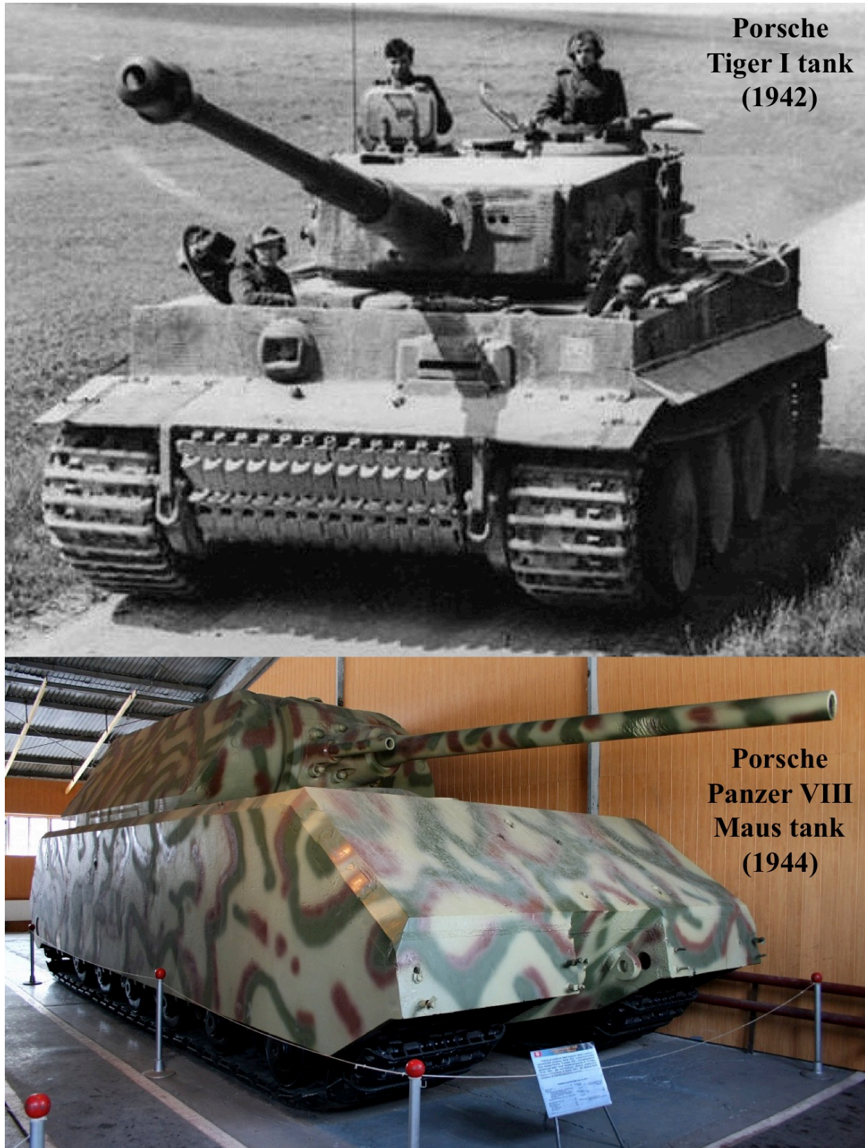
Figure 7.58: Ferdinand Porsche, Karl Rabe, and their team developed advanced tanks such as the Tiger I 57-ton tank and the Panzerkampfwagen VIII Maus prototype 188-ton tank (now in the Kubinka Tank Museum) during World War II.
