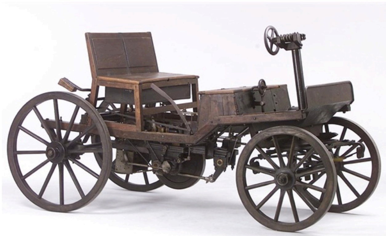
Figure 7.30: Siegfried Marcus developed an internal-combustion-engine-powered car in 1870, and a greatly improved version in 1888.
