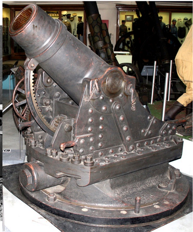
Figure 7.94: In 1880, engineers at Krupp invented the first modern mortars (Mörser), which were rifled breech-loaders designed for different calibers of ammunition: 7.5 cm, 15 cm, 21 cm, and other sizes. They could be used either mounted on a wheeled carriage or unmounted on a flat base.
