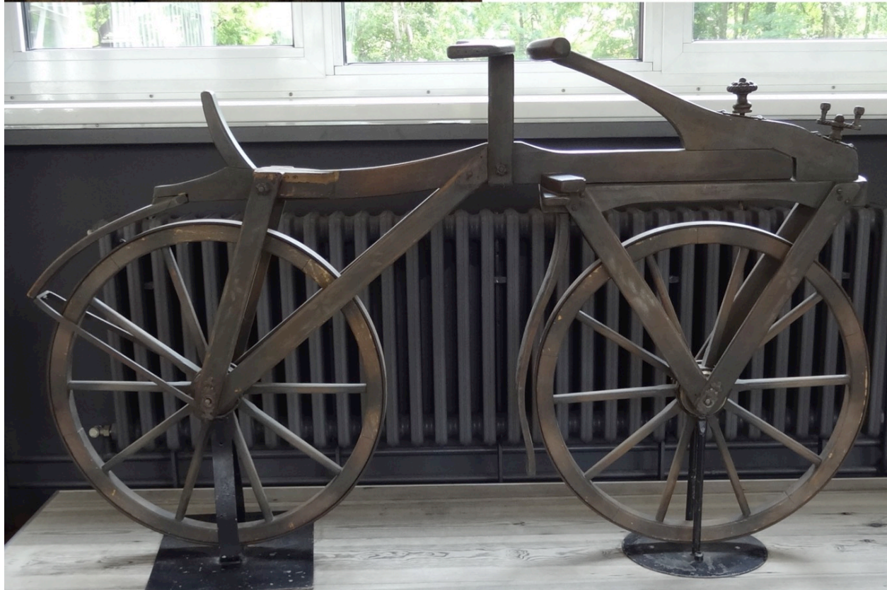
Figure 7.141: Karl von Drais invented a quadracycle with pedals in 1813, followed in 1817 by the first bicycle without pedals, which proved to be far more popular.
