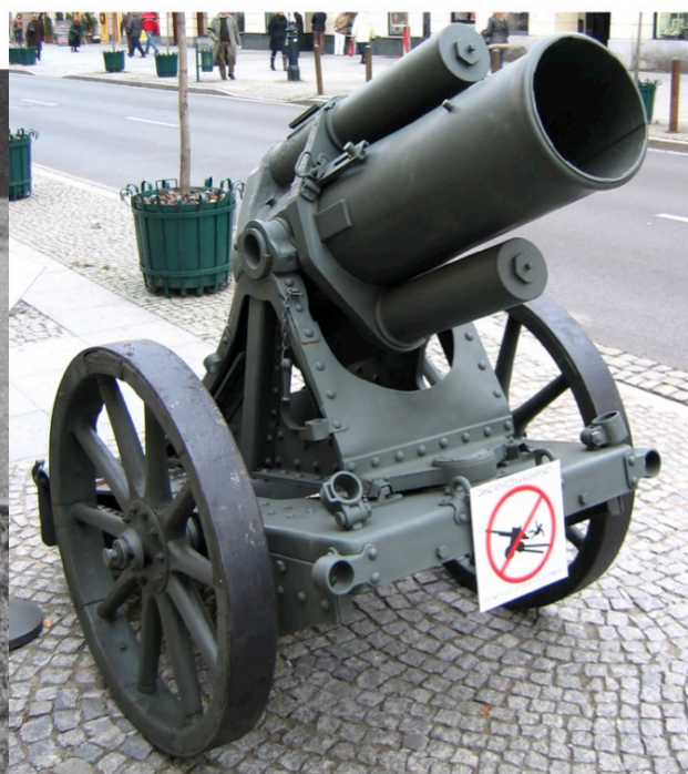
Figure 7.95: In 1909, engineers at Rheinmetall developed improved trench mortars (Mineswerfer), which were designed for three calibers of ammunition: 7.58 cm (leichte), 17 cm (mittlerer), and 25 cm (schwerer). Like the earlier Krupp mortars, all three sizes were used either mounted on a wheeled carriage or unmounted on a flat base.
