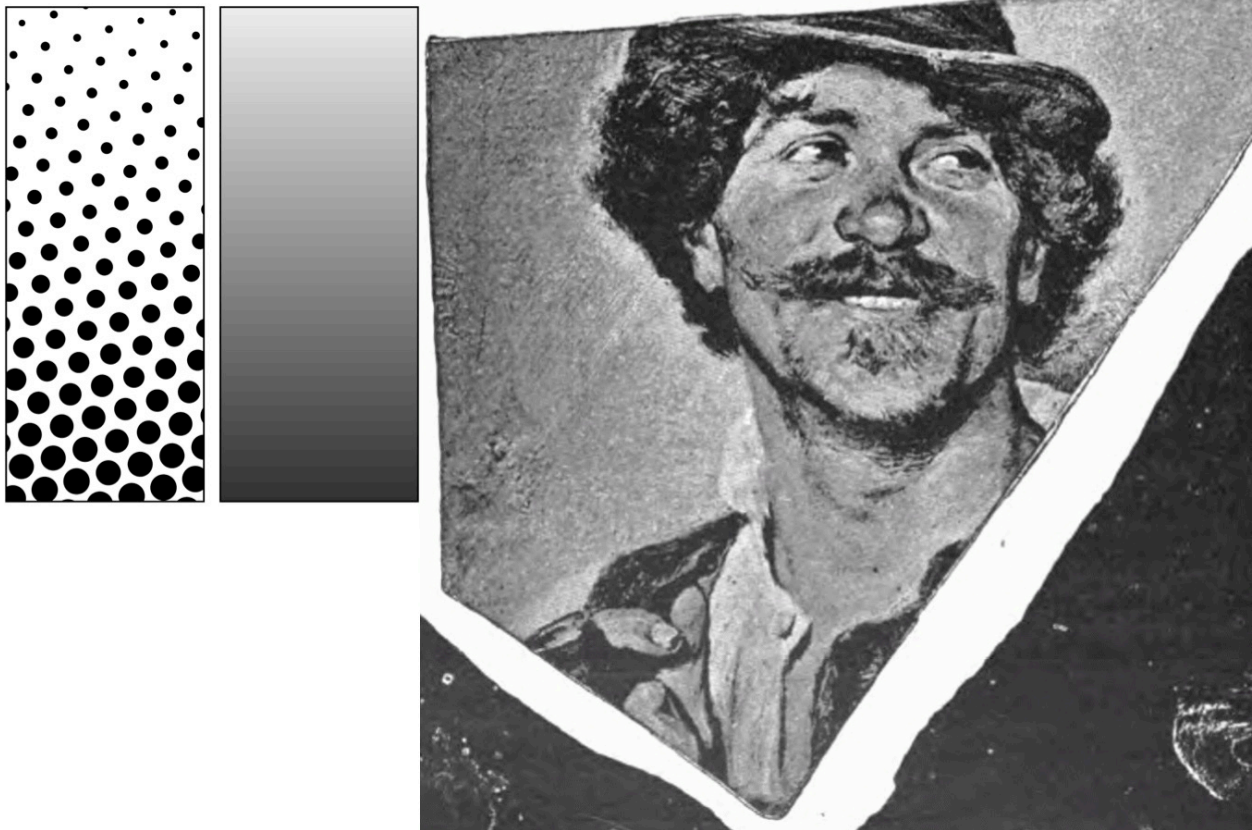
Figure 7.10: Paul Pretsch and A. J. Berchtold did early work and Georg Meisenbach perfected the halftone method for reproducing photographs with tiny printed dots.
