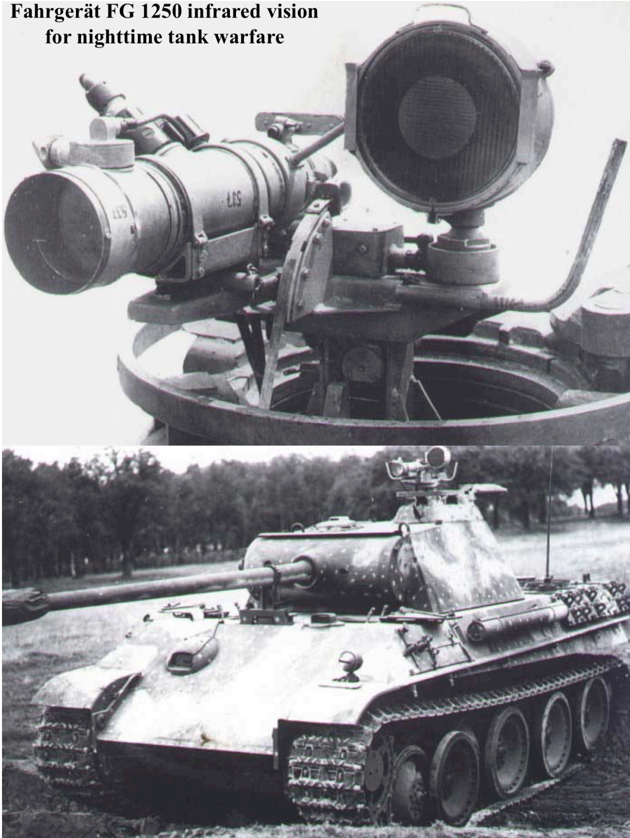
Figure 6.141: The Fahrgerät FG 1250 infrared vision system was also used for nighttime tank warfare.
