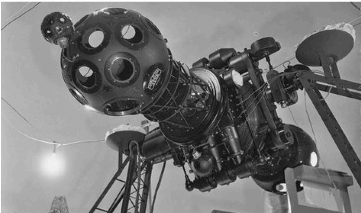
Figure 6.240: Walther Bauersfeld (1879–1959) developed the Zeiss planetarium projector Mark I (1912–1923), Mark II (1930), and later models.
