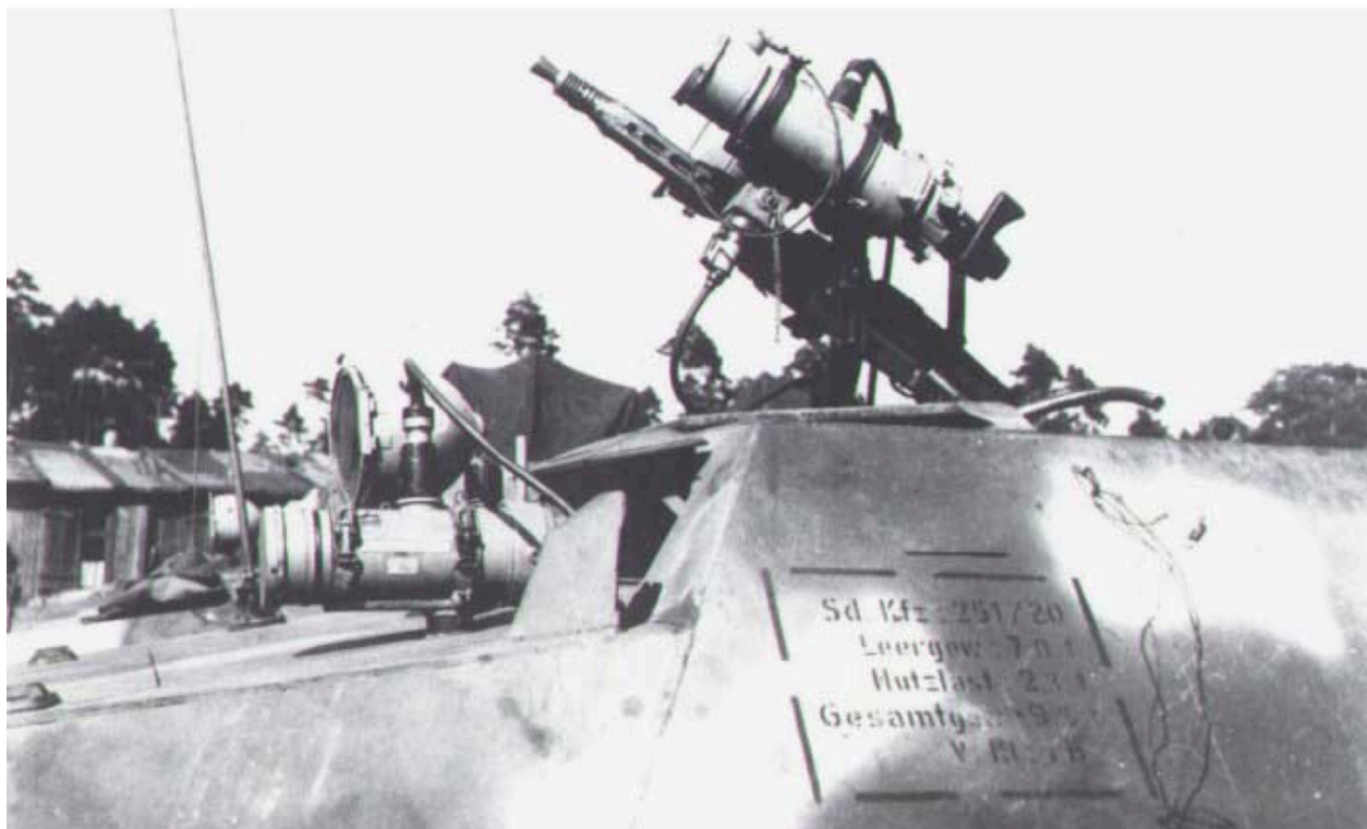
Figure 6.142: Example of an armored vehicle with two Fahrgerät FG 1250 infrared vision systems, one for a nighttime anti-aircraft gun and another for nighttime driving [BIOS Misc 66].
