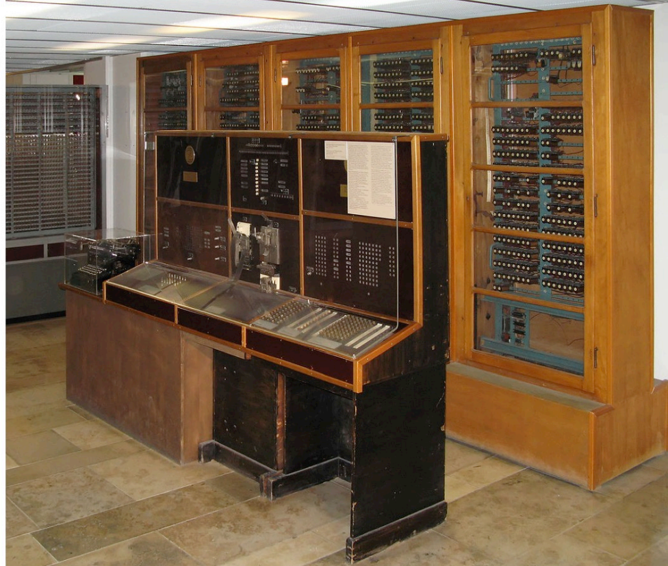
Figure 6.168: Other programmable digital computers built by Konrad Zuse included the Z3 (first operational in 1941, destroyed during the war, and rebuilt later) and the Z4 (first operational in 1944).
