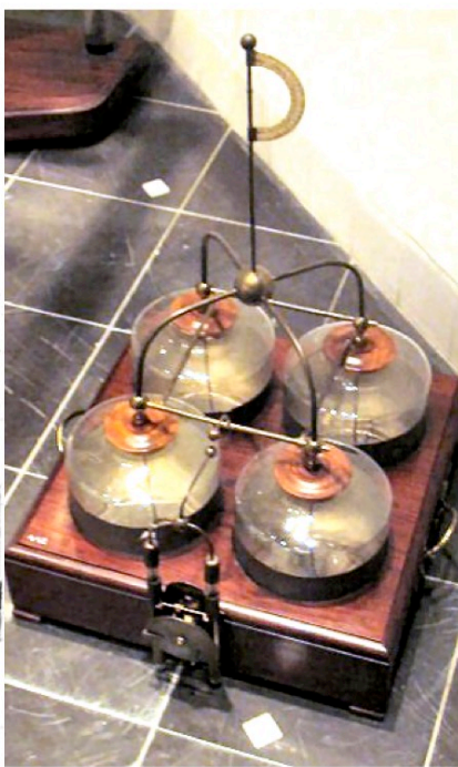
Figure 6.102: In 1745, Ewald Georg von Kleist invented the capacitor, which temporarily stores electric charge. Pieter van Musschenbroek conducted further experiments with capacitors, and they became known as “Leiden jars.” Daniel Gralath realized that multiple Leiden jars could be connected together to store more electric charge.
