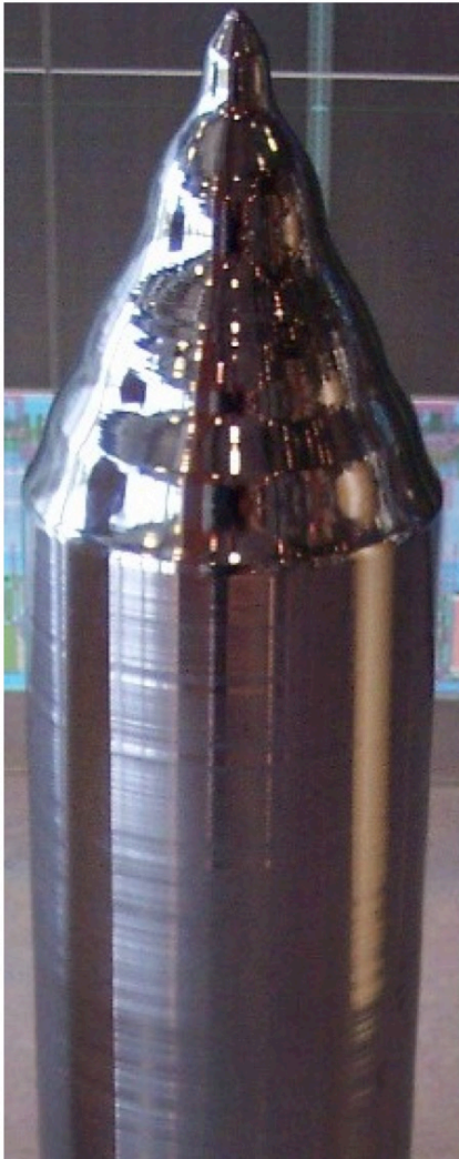
Figure 6.73: Jan Czochralski at AEG developed a method for growing semiconductor crystals and wafers in 1916.
