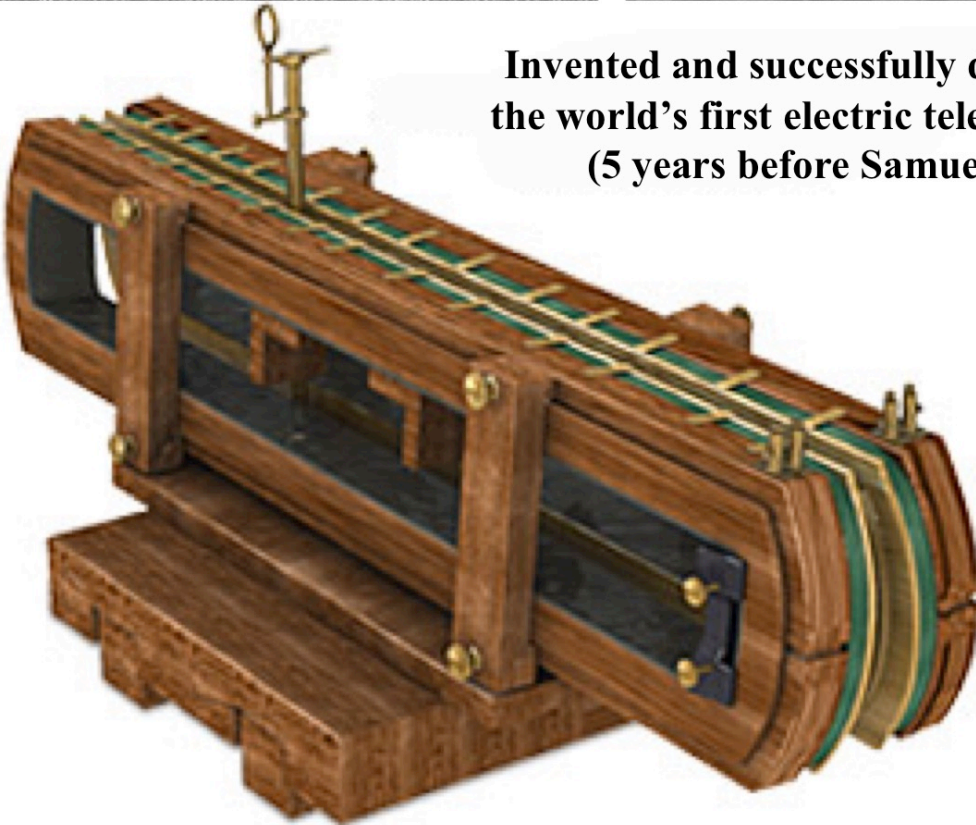
Figure 6.22: Carl Friedrich Gauss and Wilhelm Weber invented and successfully demonstrated the world's first electric telegraph in 1833 (five years before Samuel Morse).
