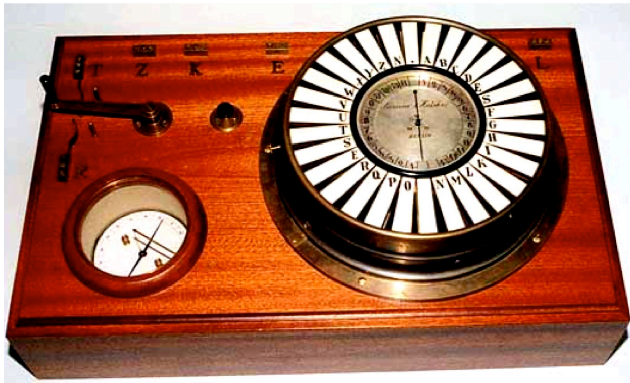
Figure 6.23: In 1846, Werner von Siemens created more sophisticated telegraphs that could point to individual letters.
