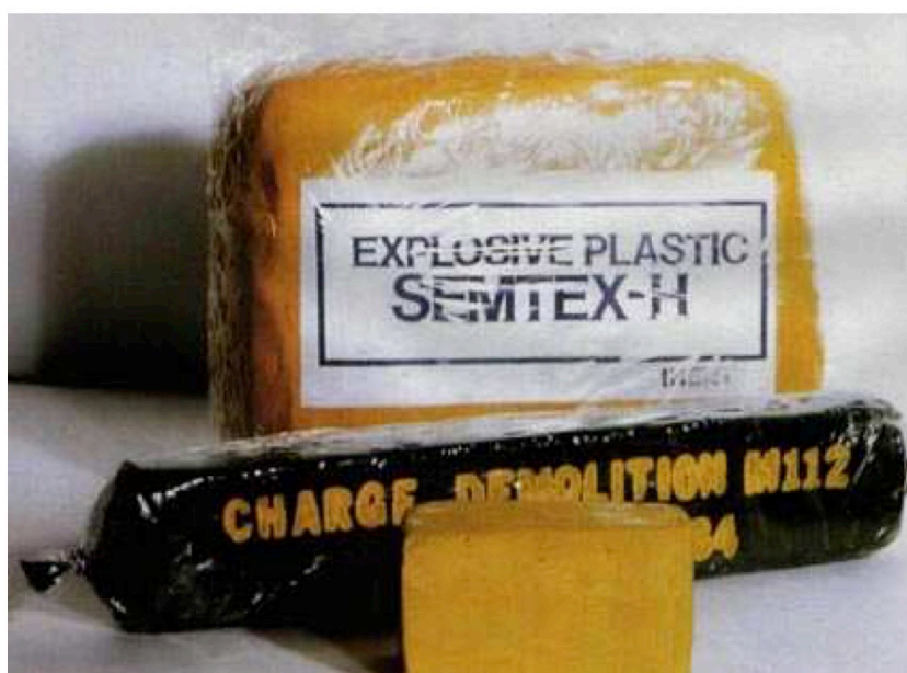
Figure 3.73: Bernhard Tollens and Peter Wigand developed pentaerythritol tetranitrate (PETN) explosive in 1891. Semtex plastic explosive is a mixture of PETN, RDX, and polymers. PETN is also used as a blood pressure medication.
