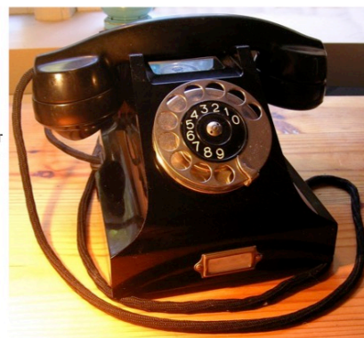
Figure 3.149: Phenol formaldehyde (phenolic) resin was first created in 1891 by Adolf von Baeyer and Werner Kleeberg, and developed further by Adolf Luft and Leo Baekeland. Phenolic resin was commercialized as Bakelite and other trade names and used to make early plastic products such as telephone cases.
