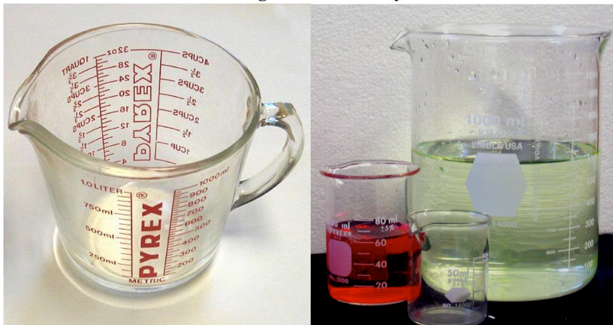
Figure 3.173: Otto Schott created optical glass, lithium glass, borosilicate glass. Borosilicate glass is resistant to thermal stress and widely used for glassware containers for cooking and laboratory work.
