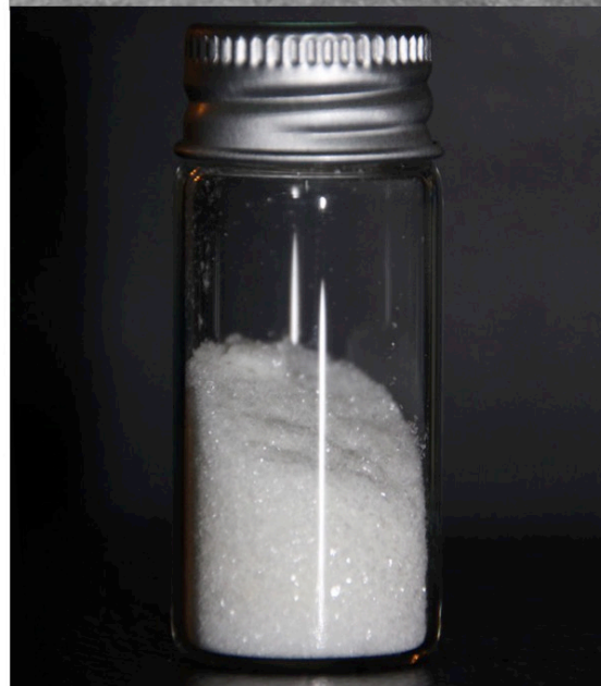
Figure 3.64: In 1935, Ferdinand Münz created the synthetic preservative ethylenediaminetetraacetic acid (EDTA), which works by chelating (trapping) metal ions that are needed by degradative enzymes and bacteria.
