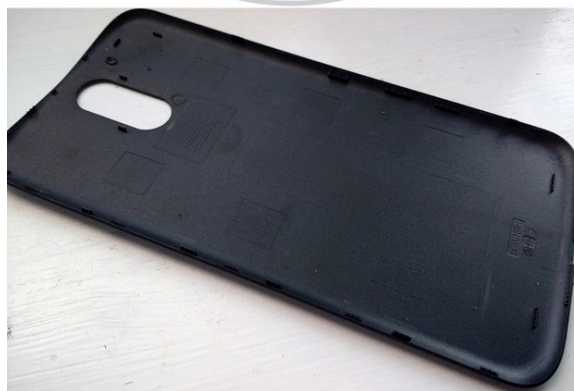
Figure 3.152: Polycarbonate was first created in 1898 by Alfred Einhorn, and developed further by Hermann Schnell. Because polycarbonate is very rugged, it is used to make products such as compact discs, water bottles, cell phone cases, and safety glasses.
