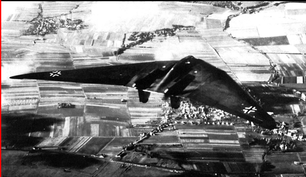
Structural materials and surface shapes that minimize radar reflections
