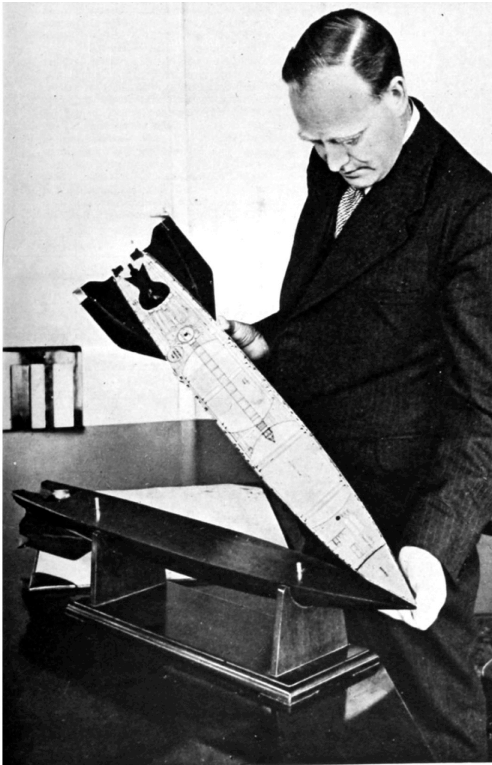
MR. W. G. A. PERRING, WITH HIS REMARKABLY ACCURATE RECONSTRUCTION OF A V-2 ROCKET, BASED ON FRAGMENTS FOUND IN SWEDEN BEFORE THE ATTACKS BEGAN. Mr. W. G. A. Perring was concerned with research work on the German V-2 rocket, and was able to make a remarkably accurate reconstruction of this weapon and assess its potentialities from some two tons of fragments found after one of these weapons had exploded over Sweden before the attacks on Britain were made. He is seen holding his diagrammatic model.
