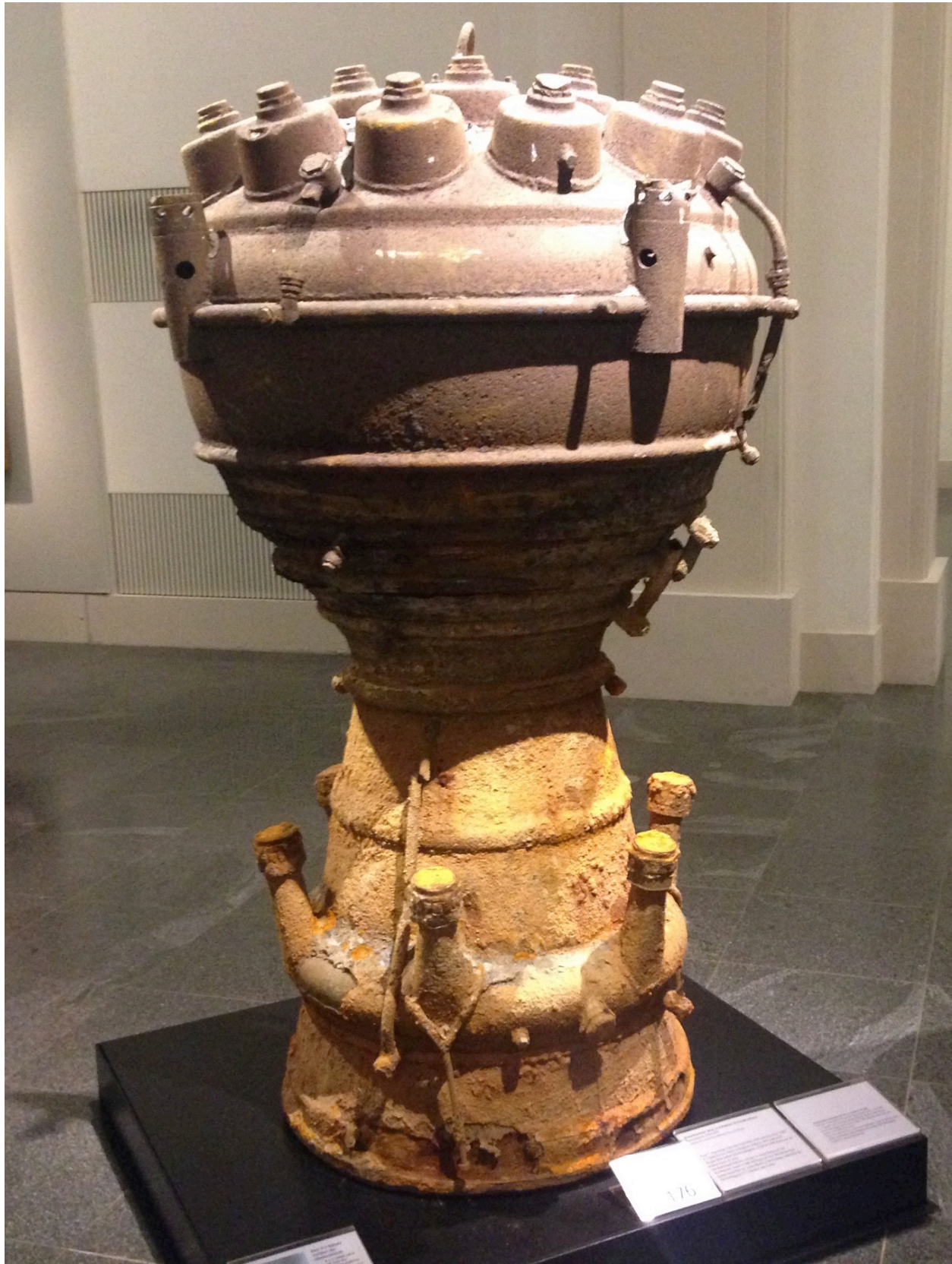
Figure E.37: Standard A-4 rocket engine with propellant injection cups on top.
