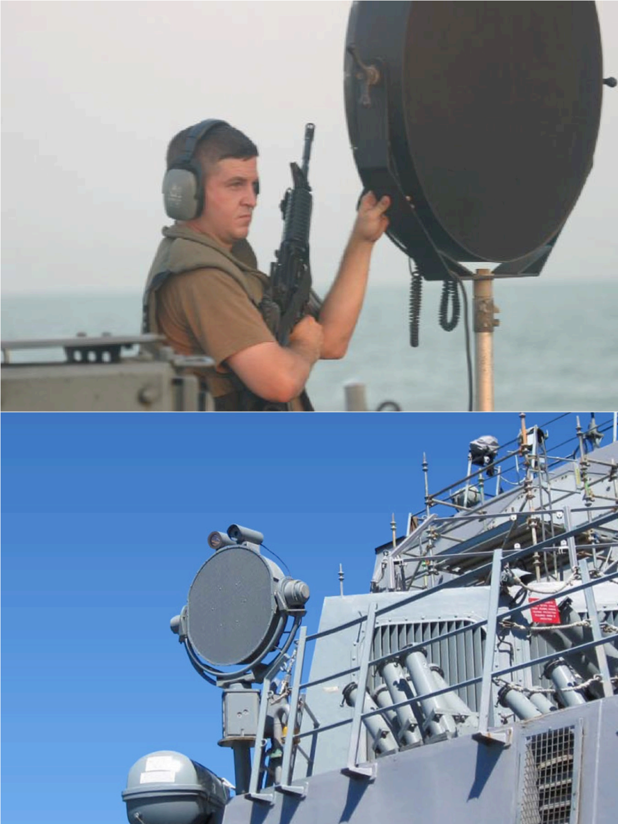
Figure C.118: Modern LRAD (Long Range Acoustic Device) acoustic weapon used by the U.S. Navy and other ships to deter pirates.
