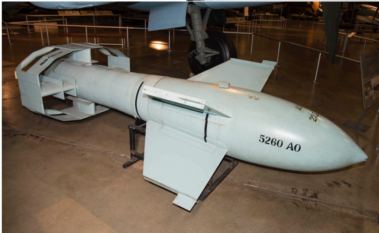
Figure 9.155: Max Kramer created precision guided weapons such as the Ruhrstahl SD 1400 X (Fritz X) radio-guided smart bomb, first operational in 1943, and the Ruhrstahl X-4 air-to-air guided missile in 1944.
