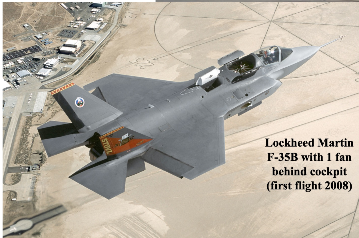
Figure 9.96: Beginning in 1957, Peter Kappus filed several patent applications on VTOL aircraft with downward-pointing fans in the wings and/or body (see also Fig. 9.97). That approach was successfully implemented in aircraft such as the Ryan XV-5 Vertifan (first flight 1964) and the Lockheed Martin F-35B (first flight 2008).
