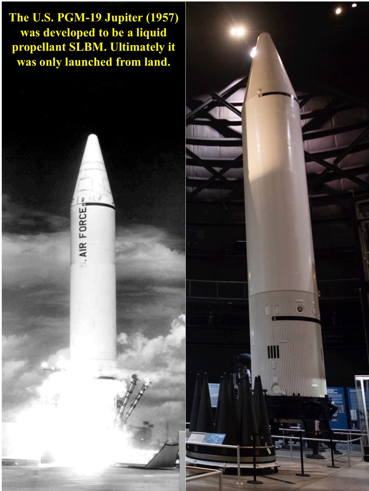
Figure 9.196: The U.S. PGM-19 Jupiter, first launched in 1957, was developed to be a liquid propellant SLBM. Ultimately it was only launched from land.
