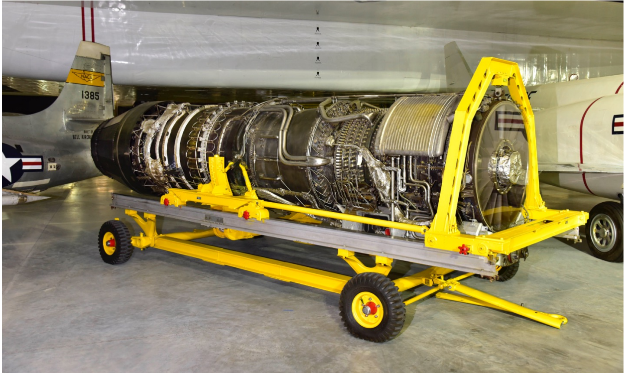
Bruno Bruckmann designed the YJ-93 engines for the Mach 3+ XB-70 Valkyrie (first flight 1964)
