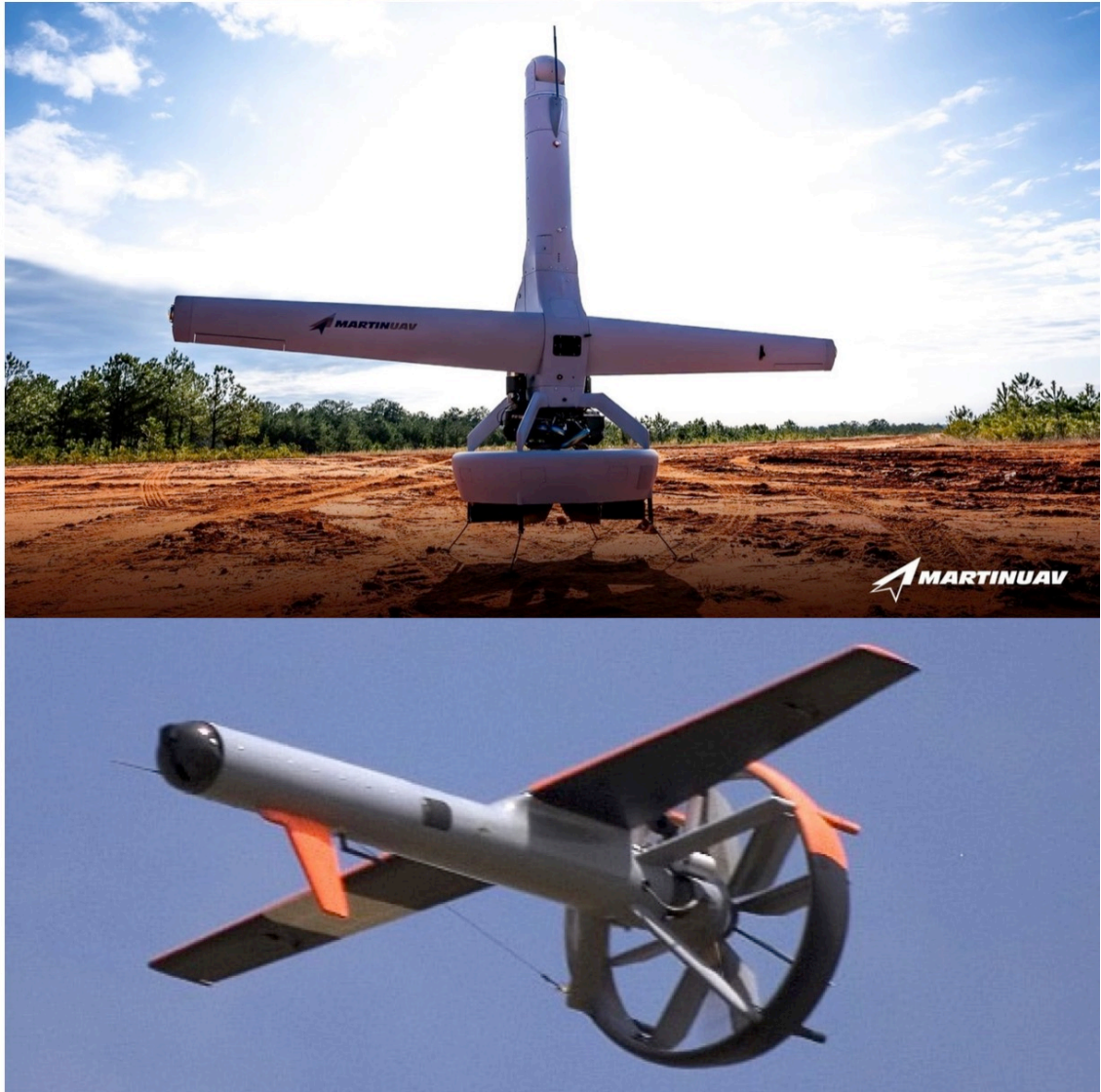
Figure 9.142: The wartime German Lerche/Wespe- and Triebflügel-type designs (for aircraft that could take off and land on their tails but pitch over by 90^\circ to fly horizontally) still live on in modern unmanned aerial vehicles (UAVs) such as the University of Kansas XQ-138 drone and the Martin UAV V-BAT drone.
