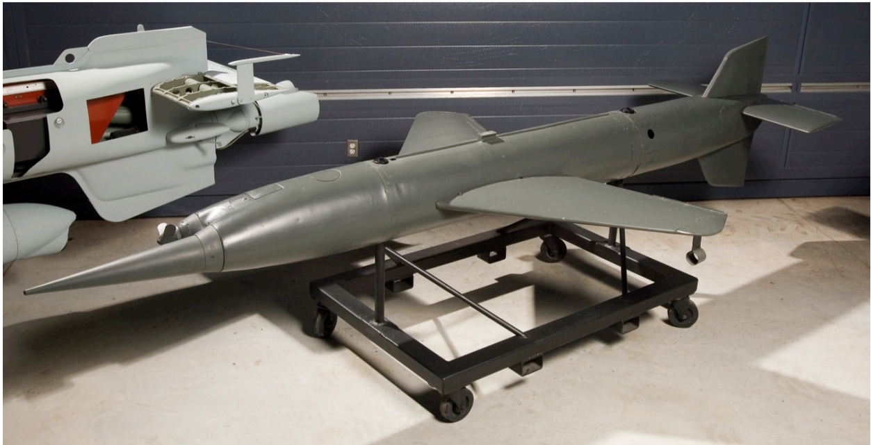
Figure 9.154: Herbert Wagner created precision guided weapons such as the Henschel Hs 293 smart bomb, first demonstrated in 1942, and the Henschel Hs 117 Schmetterling (Butterfly) surface-to-air and air-to-air missile, first demonstrated in 1944. Some versions of these weapons were guided by a miniaturized onboard camera (pp. 1008–1010).
