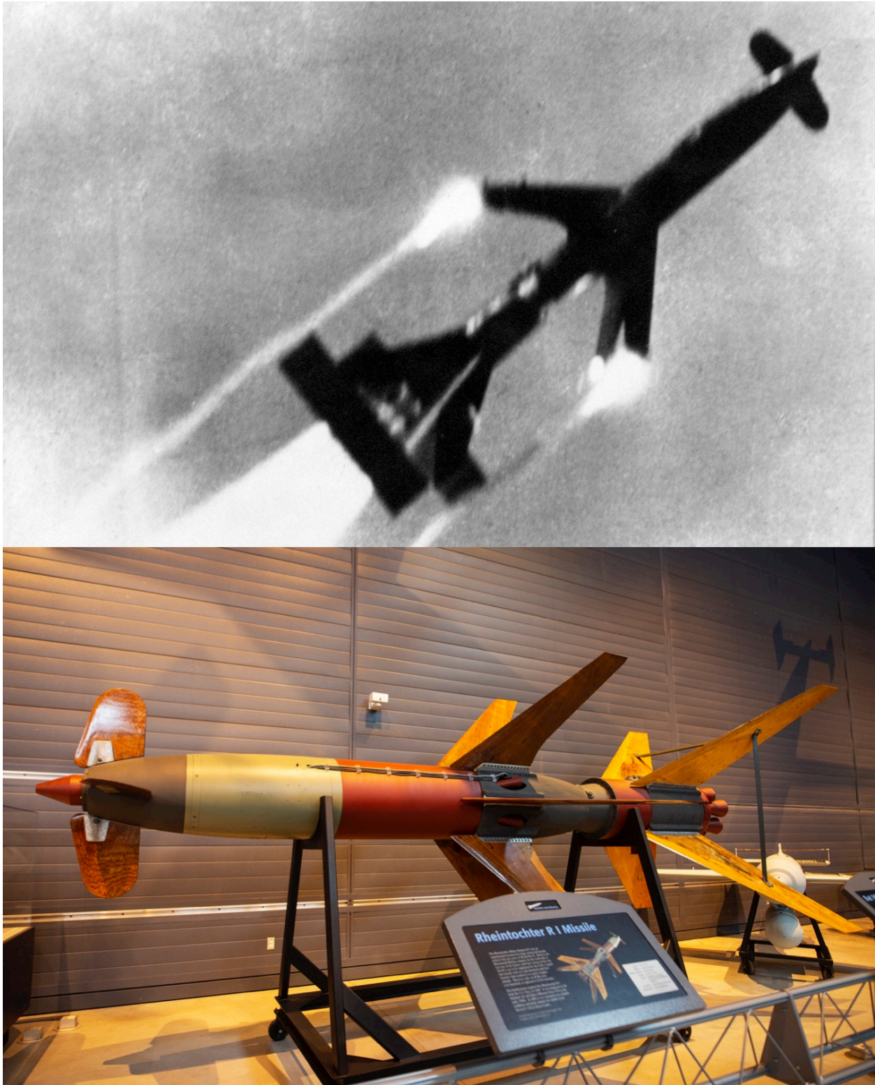
Figure 9.207: Heinrich Klein led the Rheinmetall-Borsig team that created the Rheintochter solid propellant, two-stage, surface-to-air missile, which was first launched in 1943.
