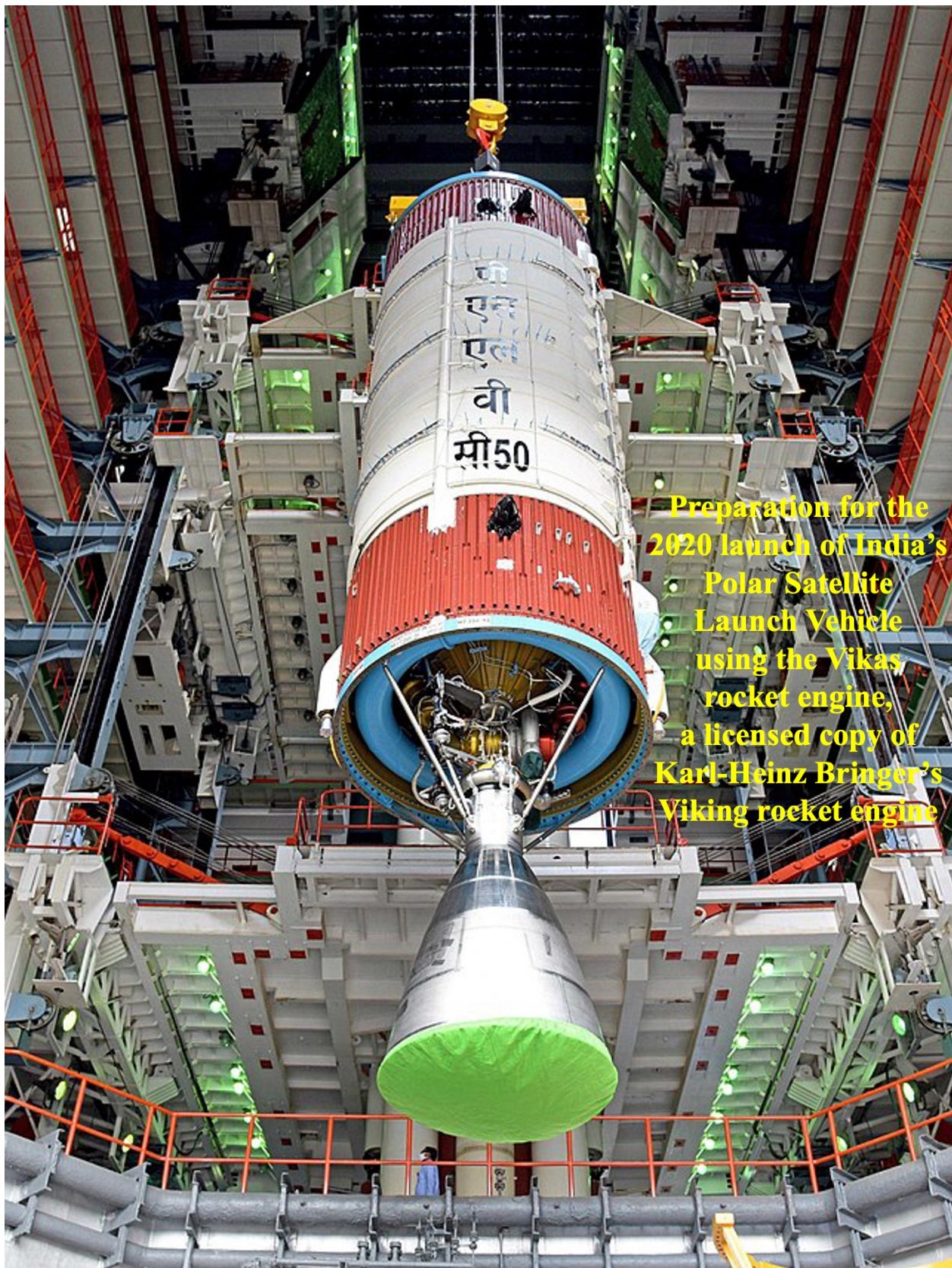
Figure 9.190: Preparation for the 2020 launch of India's Polar Satellite Launch Vehicle using the Vikas rocket engine, a licensed copy of Karl-Heinz Bringer's Viking rocket engine, as well as other German-designed Ariane technologies. See also: https://www.b14643.de/Spacerockets/Specials/VIKAS_engines/Vikas.htm
