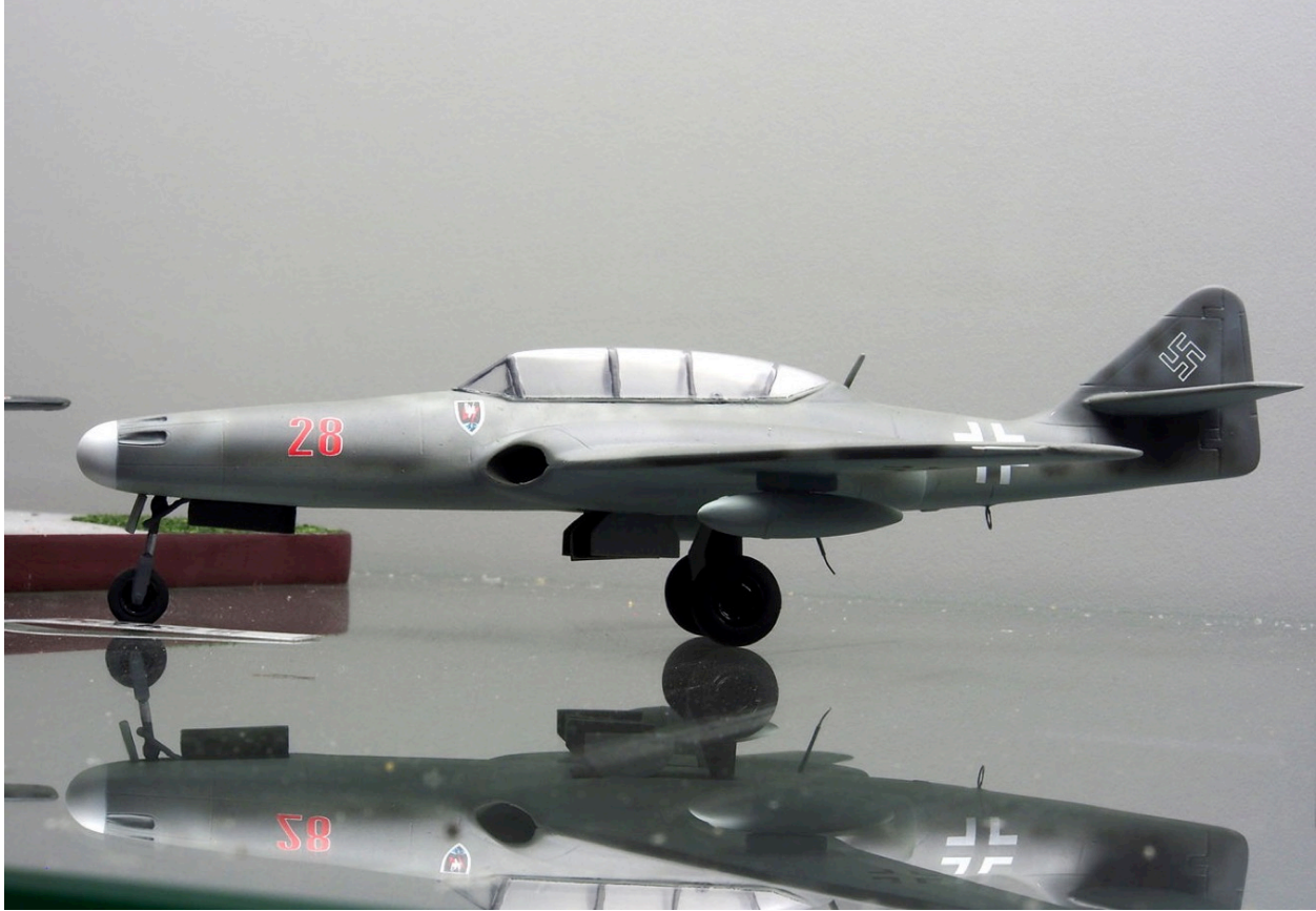
Figure 9.103: An upgraded version of the Messerschmitt Schwalbe with integrated jet engines and a two-person cockpit, Me 262 HG III, was designed but apparently not built before the end of the war.
