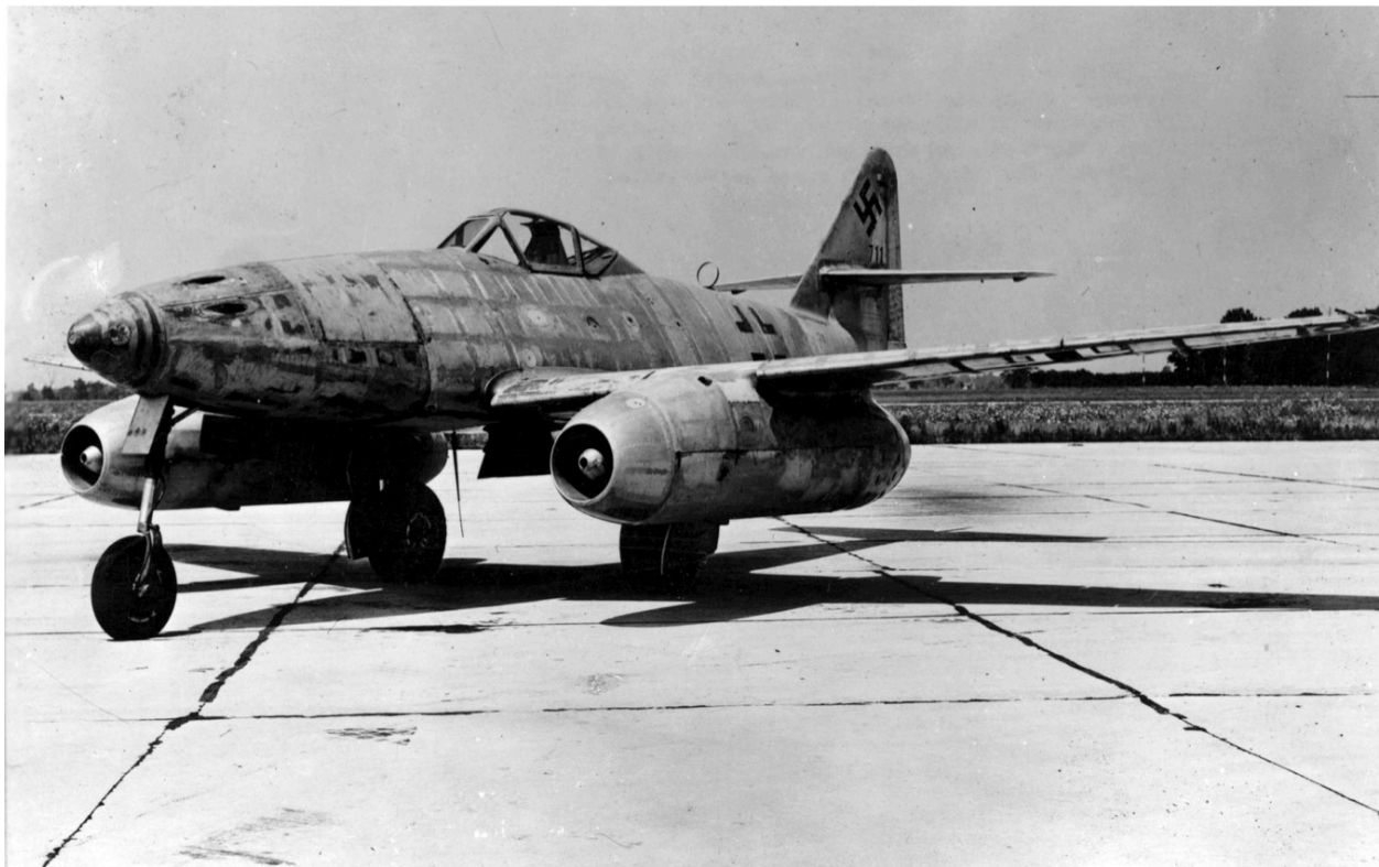
Figure 9.102: Willy Messerschmitt, Ludwig Bölkow, and Woldemar Voigt headed the team that developed and mass-produced the Messerschmitt Me 262 Schwalbe (Swallow) twin-engine jet fighter, which was first flown in 1942.
