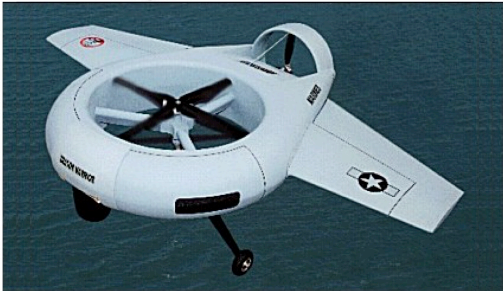
Figure 9.138: In 1939, Henrich Focke and his team designed the Rothen, a winged VTOL aircraft with counter-rotating rotors in a ducted fan. Focke's design lives on in examples such as the Sikorsky Cypher II or Dragon Warrior drone (2000).
