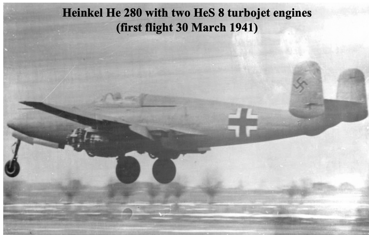
Figure 9.68: Top: HeS 8 turbojet engine (first run September 1940). Bottom: Heinkel He 280 with two HeS 8 turbojet engines (first flight 30 March 1941).
