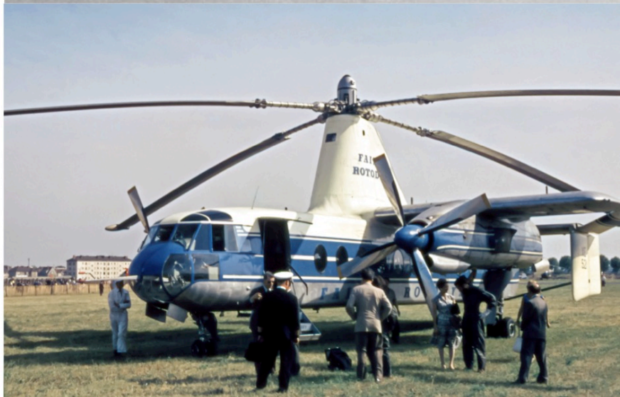
Figure 9.147: After the war, members of Friedrich von Doblhoff's team continued to develop helicopters propelled by tip-jet rotors, such as the McDonnell XV-1 military helicopter, Fairey Jet Gyrodyne test prototype, and Fairey Rotodyne passenger vehicle.
