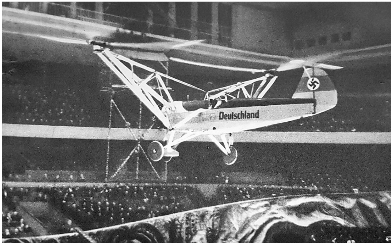
Figure 9.132: Henrich Focke and his team, including Walter Just and Paul Klages, created the world's first fully functional helicopter, the Focke-Wulf Fw 61, in 1936. In 1938, test pilot Hanna Reitsch (Fig. 9.217) demonstrated the Fw 61 in a crowded indoor arena in Berlin.
