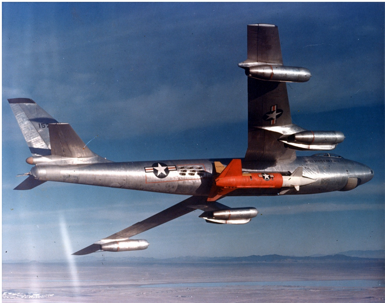
Figure 9.164: The Bell GAM-63 RASCAL air-launched cruise missile was designed by Walter Dornberger in 1946 and first launched in 1953. Essentially it was a German-derived liquid propellant rocket that was intermediate in size between the Wasserfall (p. 1844) and A-4/V-2 (p. 1860) and was deployed like the air-launched V-1 (p. 1841).
