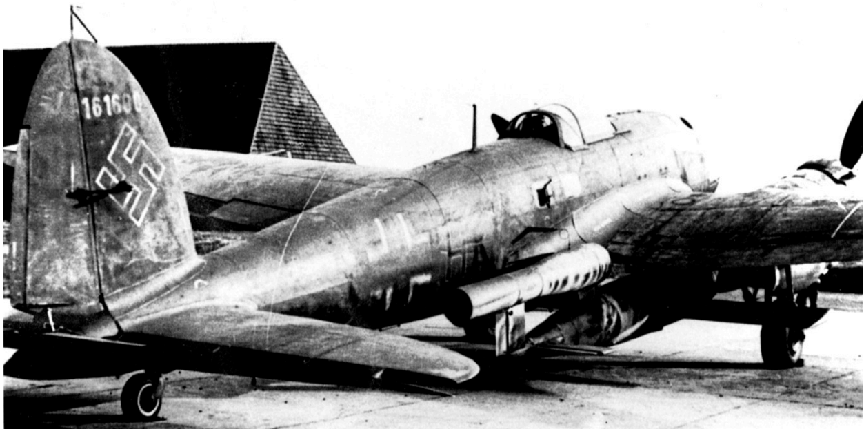
Figure 9.153: During the war, versions of the V-1 cruise missile that were piloted and/or air-launched were also produced and demonstrated.
