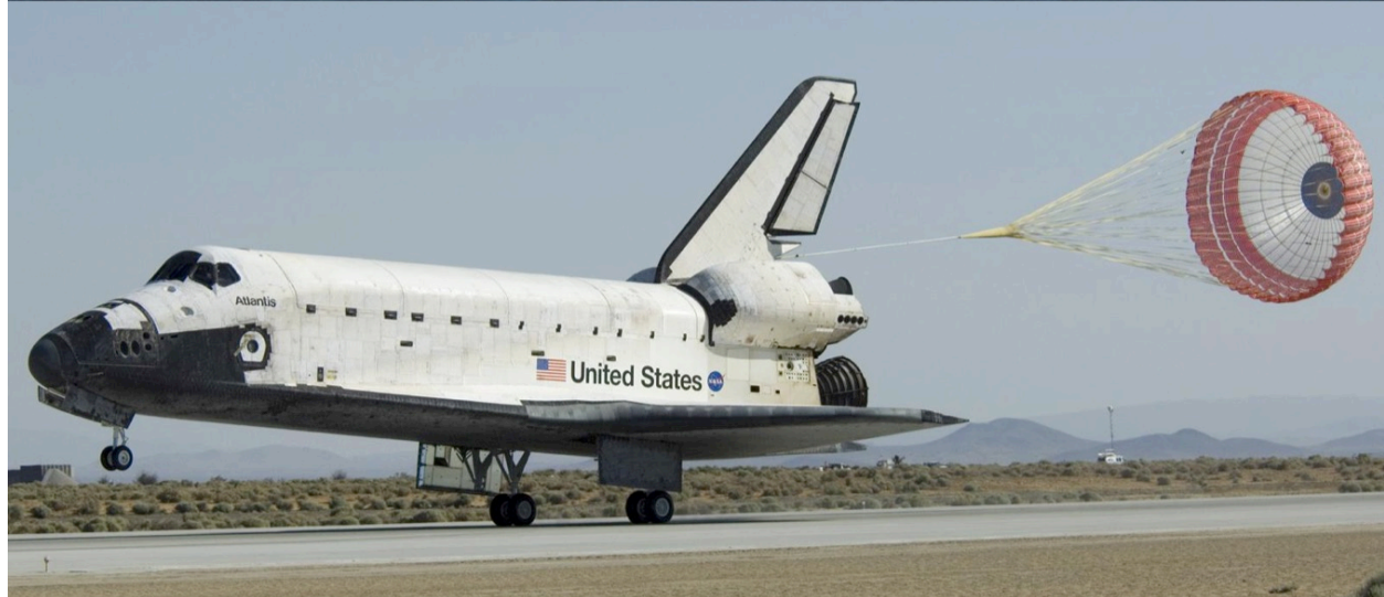
Figure 9.117: German-designed auxiliary parachutes, ribbon braking parachutes, and other specialized parachutes have been widely used in aerospace applications ranging from Apollo capsules to the Space Shuttle.
