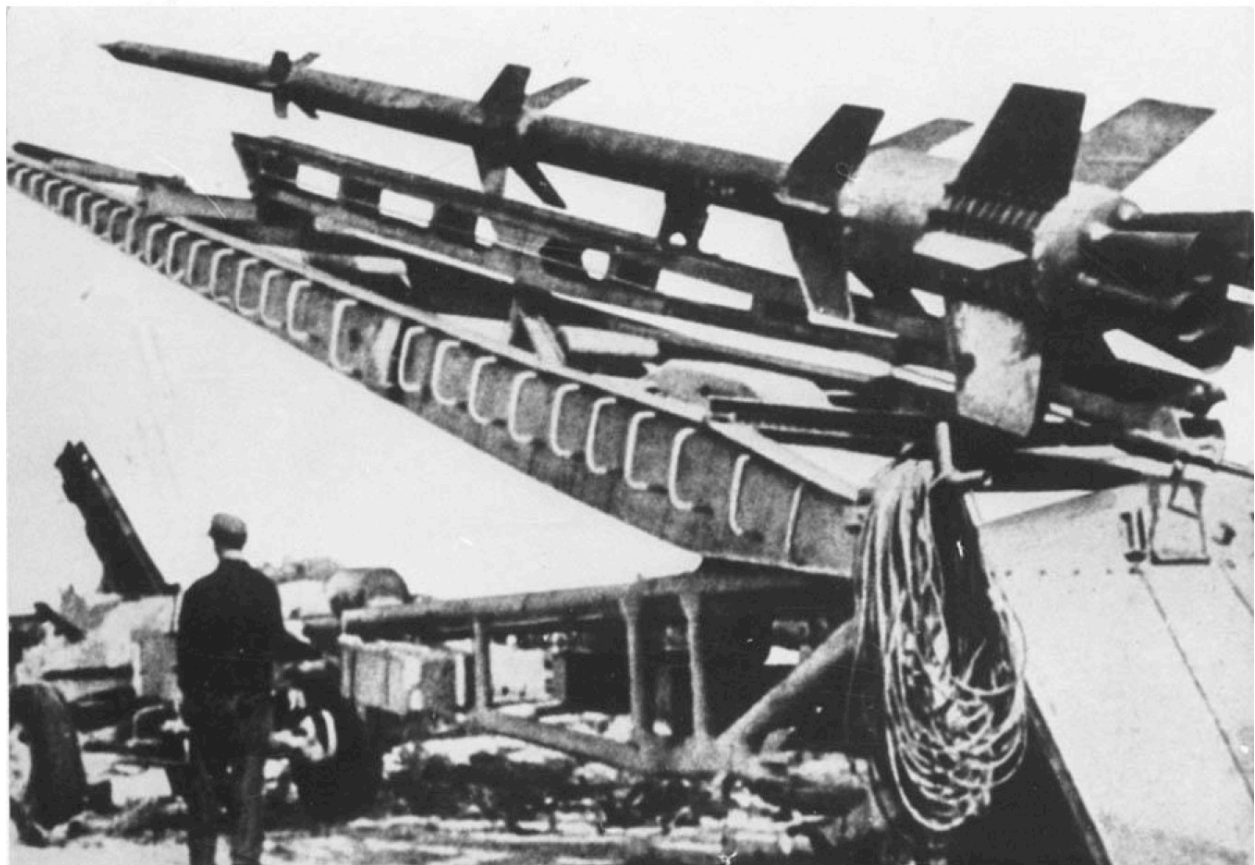
Figure 9.208: Heinrich Klein and his Rheinmetall-Borsig team also created the Rheinbote solid propellant, four-stage, long-range rocket, which was first launched in 1943.
