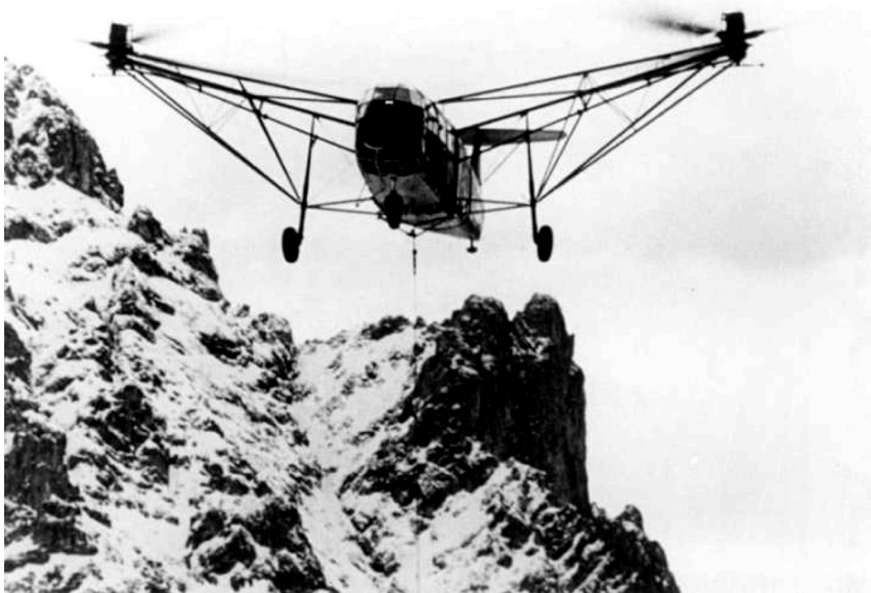
Figure 9.133: Henrich Focke and his team created the much more advanced Focke-Achgelis Fa 223 Drache (Dragon) dual-rotor cargo helicopter in 1940.
