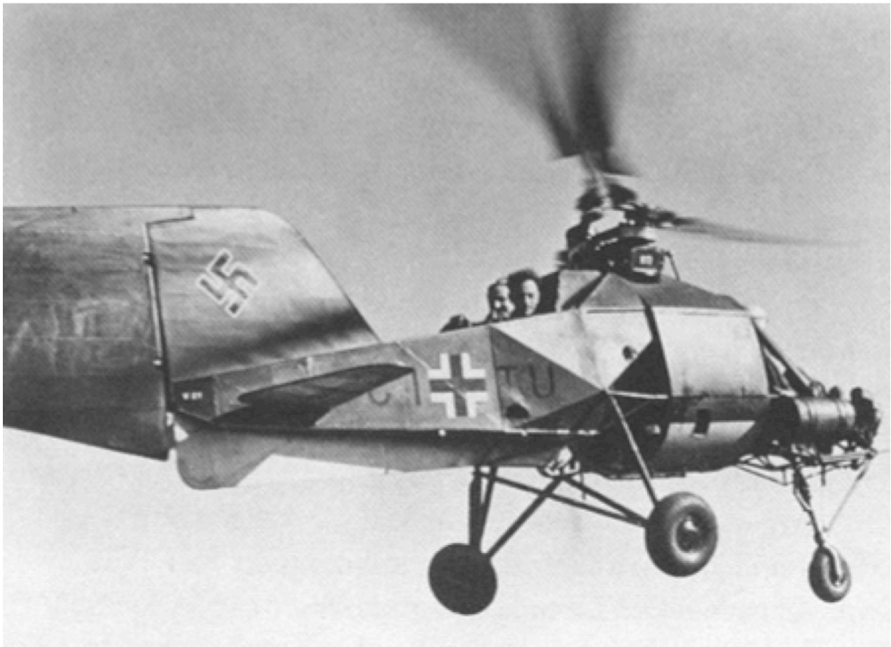
Figure 9.144: Anton Flettner and his team produced the much more advanced Fl 282 Kolibri (Humming Bird) reconnaissance helicopter in 1941.
