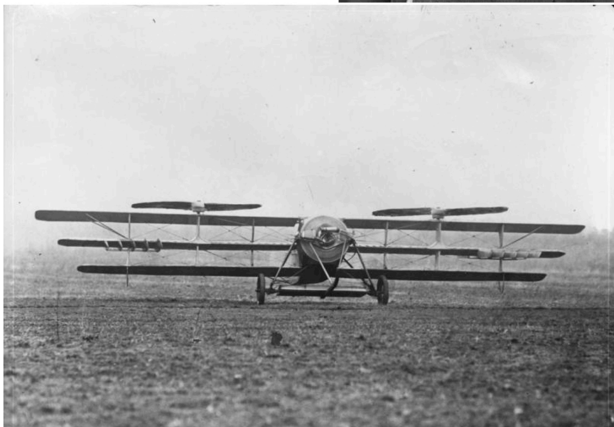
Figure 9.126: Emil Berliner created proto-helicopters and autogyros such as the Berliner Helicopter No. 5 (1923).
