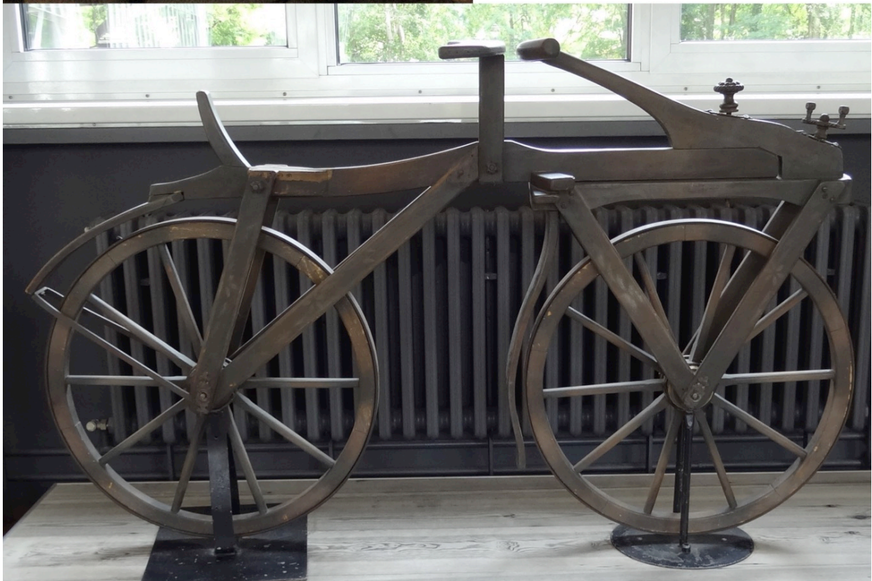
Figure 7.140: Karl von Drais invented a quadracycle with pedals in 1813, followed in 1817 by the first bicycle without pedals, which proved to be far more popular.
