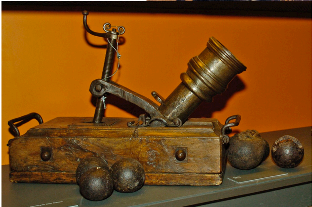
Figure 7.92: In 1674, Menno van Coehoorn invented the Coehoorn or Coehorn style of mortar, which was widely used until the early twentieth century. He also made other innovations in methods of attacking or defending fortifications.
