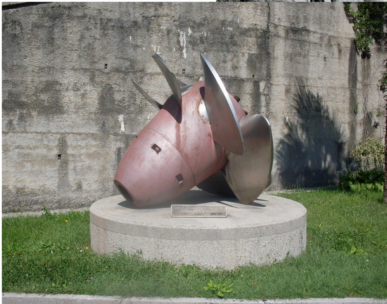
Figure 7.144: Viktor Kaplan invented highly efficient turbines with blades of adjustable tilt for hydroelectric power. See also p. 3757.
