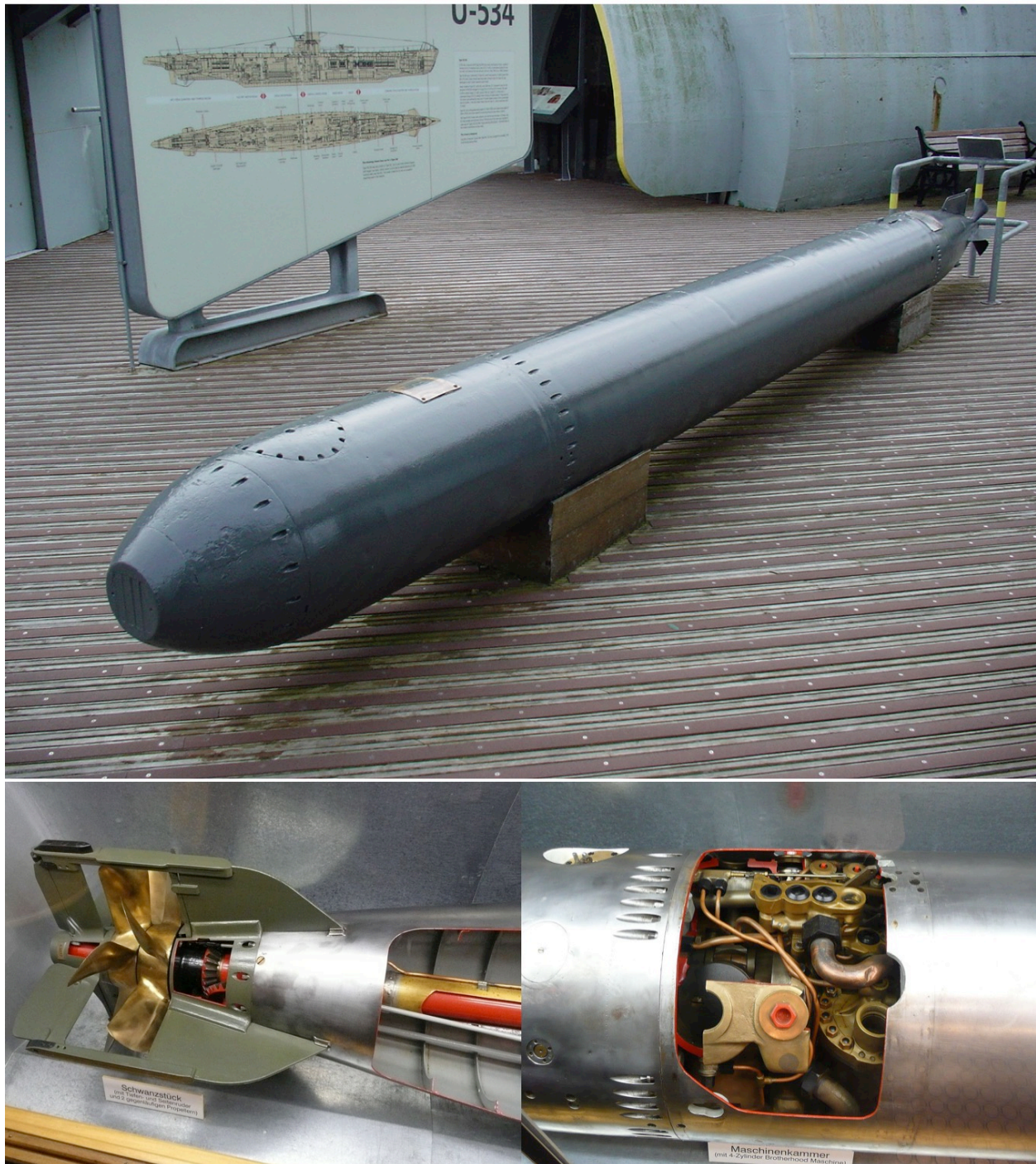
Figure 7.127: Some German innovations in torpedo design included improved energy sources such as batteries (in G7e torpedoes) and concentrated hydrogen peroxide ( H_2O_2 , called Ingolene). Other innovations included improved guidance systems such as preprogrammed pattern running systems (Fat I/II and Lut I/II) and acoustic homing systems (Falke and Zaunkönig).
