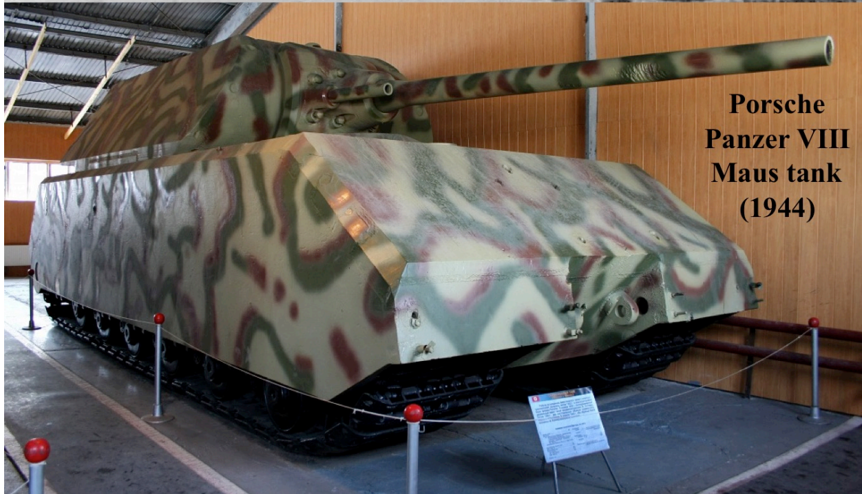
Figure 7.57: Ferdinand Porsche, Karl Rabe, and their team developed advanced tanks such as the Tiger I 57-ton tank and the Panzerkampfwagen VIII Maus prototype 188-ton tank (now in the Kubinka Tank Museum) during World War II.
