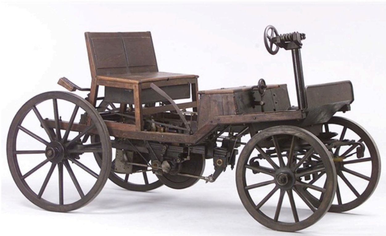
Figure 7.29: Siegfried Marcus developed an internal-combustion-engine-powered car in 1870, and a greatly improved version in 1888.
