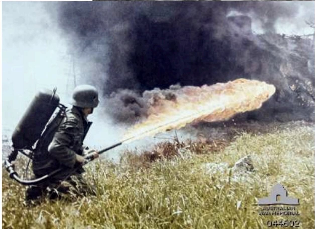
Figure 7.105: The one-person portable Flammenwerfer 35 (1935) weighed 36 kilograms and had a range of 25 meters.
