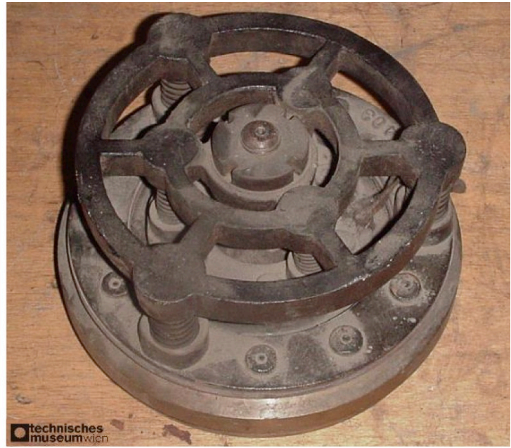
Hörbiger disc valve for high-pressure chemistry, compressors, etc. (1894)
