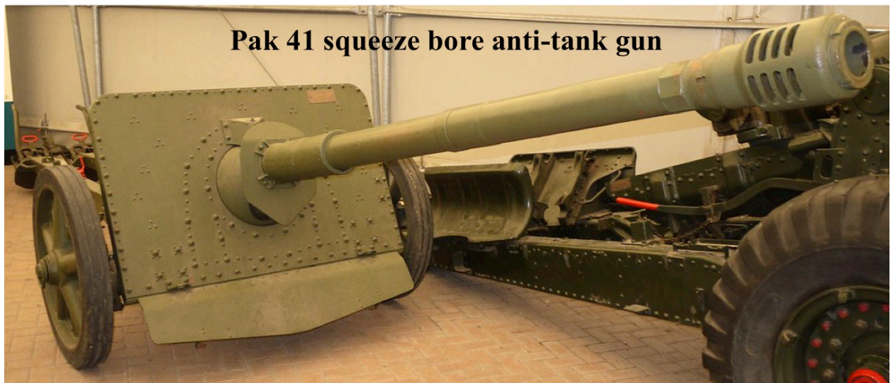
Figure 7.101: Karl Puff patented a squeeze bore or tapered bore gun design for increasing muzzle velocities in 1904. Hermann Gerlich filed more detailed patent applications in 1929 and built such guns. The German military used squeeze bore guns such as the Pak 41 anti-tank gun (1941).
