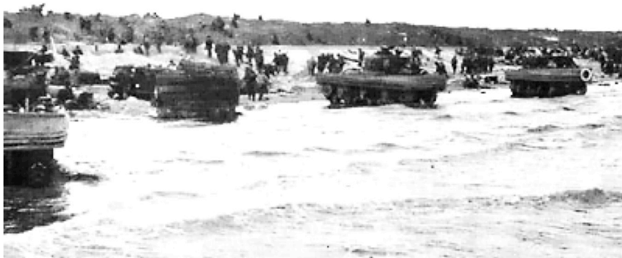
Figure 7.59: Nicholas Straussler emigrated to the United Kingdom and developed the duplex drive (DD) amphibious tanks that were used by Allied forces for the invasion of Normandy.
