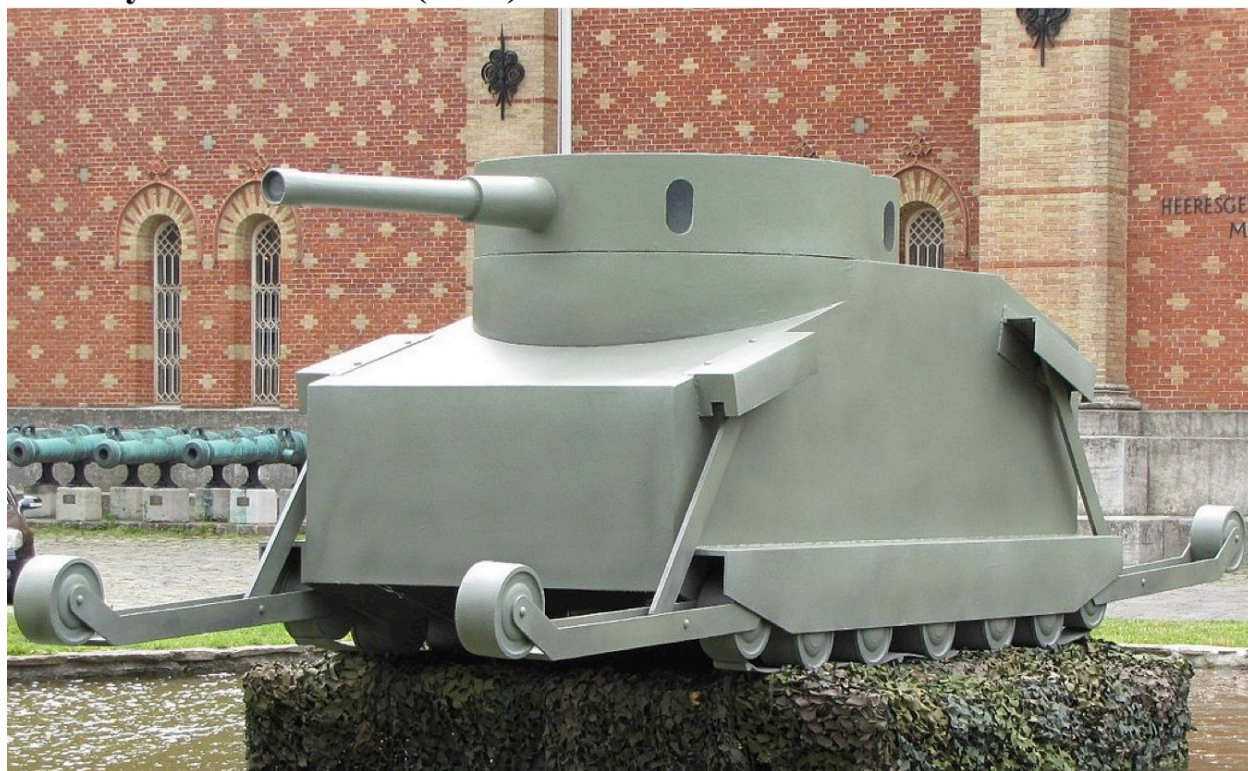
Figure 7.53: In or before 1911, Günther Burstyn invented the first combat tank to incorporate all of the major features of modern tanks. It also had extendable wheeled beams on the front and back to aid in crossing over trenches.
