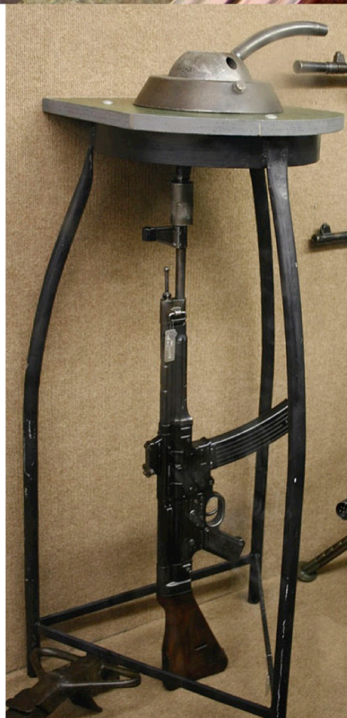
Figure 7.91: The Krummlauf (curved barrel) modified Sturmgewehr 44 could shoot around corners, and was equipped with a periscope for seeing around corners (1944). Krummlauf rifles were also installed in tank ports to defend the exterior of tanks from close attackers.
