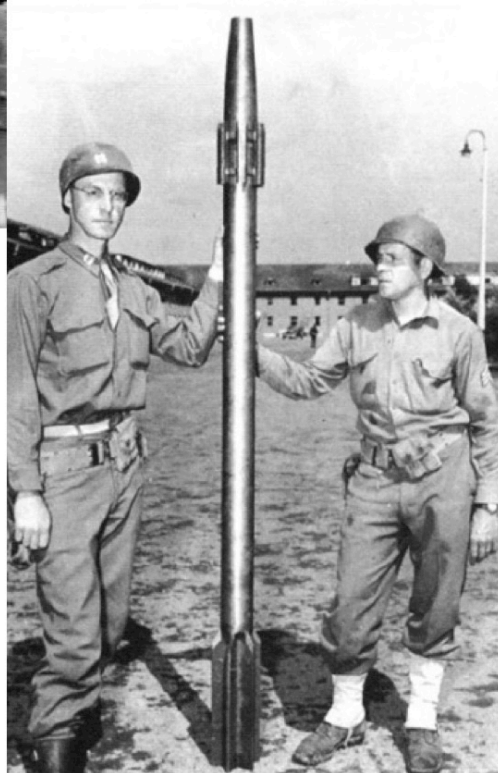
Figure 7.100: In 1944, engineers at Krupp demonstrated the Hochdruckpumpe or “V-3” gun, which could fire projectiles with a mass of 140 kg and a caliber of 15 cm up to a maximum range of 165 km.
