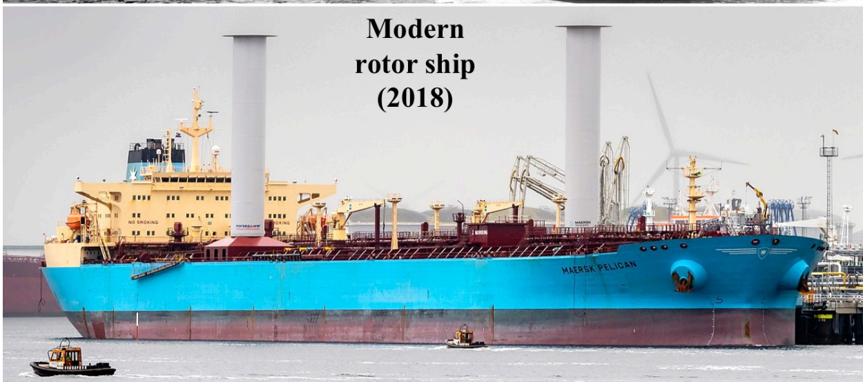
Figure 7.134: Based on the Magnus effect, Anton Flettner developed rotor ships that use spinning cylinders like sails for steering or propulsion. Flettner demonstrated the first rotor ship in 1924; rotors are still used on ships to supplement other methods and increase energy efficiency.
