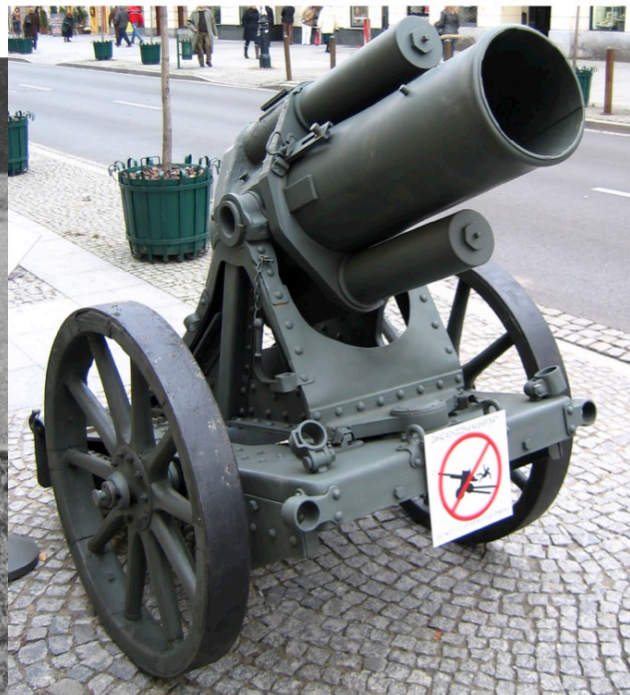
Figure 7.94: In 1909, engineers at Rheinmetall developed improved trench mortars (Mineswerfer), which were designed for three calibers of ammunition: 7.58 cm (leichte), 17 cm (mittlerer), and 25 cm (schwerer). Like the earlier Krupp mortars, all three sizes were used either mounted on a wheeled carriage or unmounted on a flat base.
