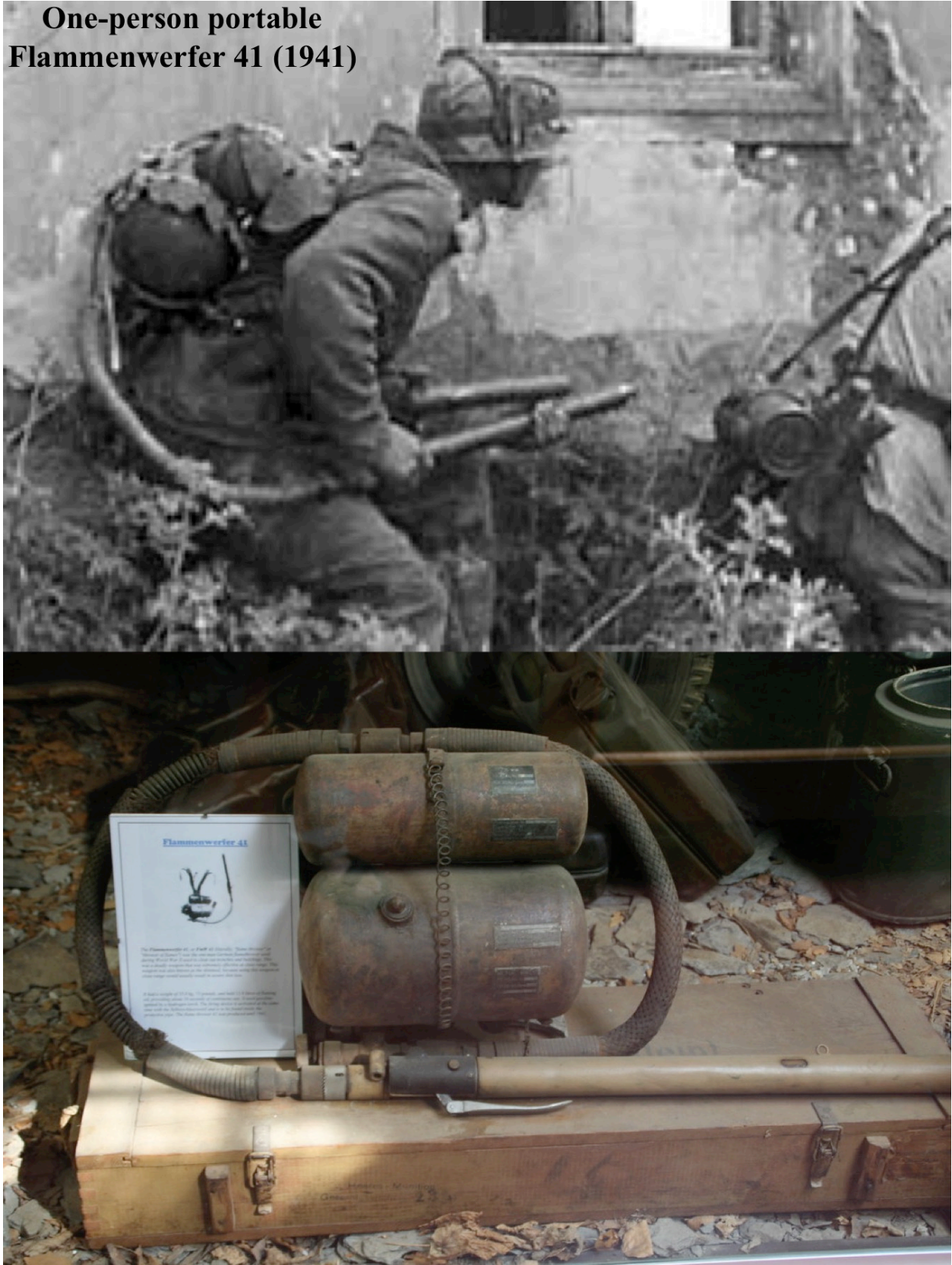
Figure 7.106: The one-person portable Flammenwerfer 41 (1941) weighed 29 kilograms and had a range of 32 meters.
