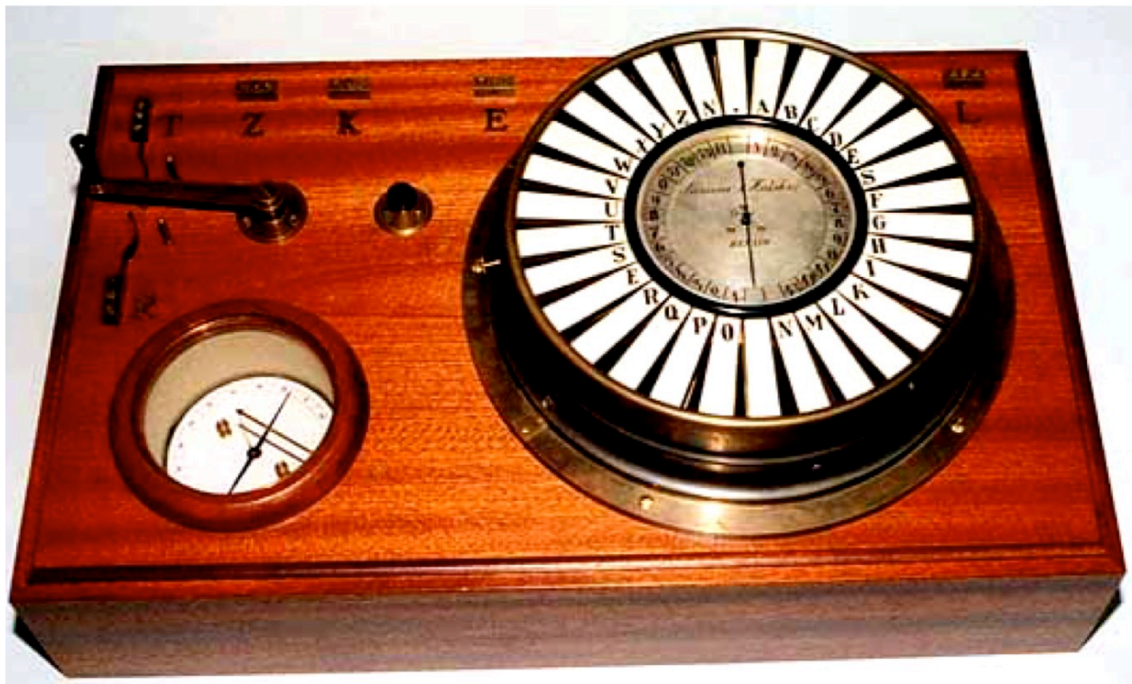
Figure 6.22: In 1846, Werner von Siemens created more sophisticated telegraphs that could point to individual letters.
