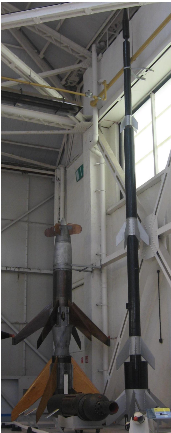
Figure E.212: Rheintochter R1 two-stage solid propellant rocket (left), partial Rheintochter R3 strap-on solid propellant booster (horizontal, center), and Rheinbote four-stage solid propellant rocket (right).
