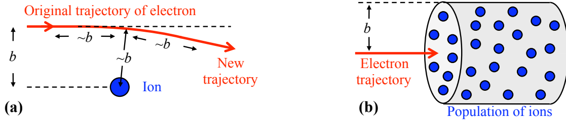
Figure 3. Bremsstrahlung radiation. (a) Due to attraction by an ion, an electron is deflected from its original trajectory to a new trajectory. If the impact parameter of the original trajectory is b , the distance of closest approach may be approximated as \sim b , and the path length over which the acceleration (trajectory deflection) occurs may be taken as \sim 2b . The acceleration causes the electron to emit bremsstrahlung radiation. (b) Acceleration of an electron by all ions may be taken into account by considering the ion density and integrating over all impact parameters.
